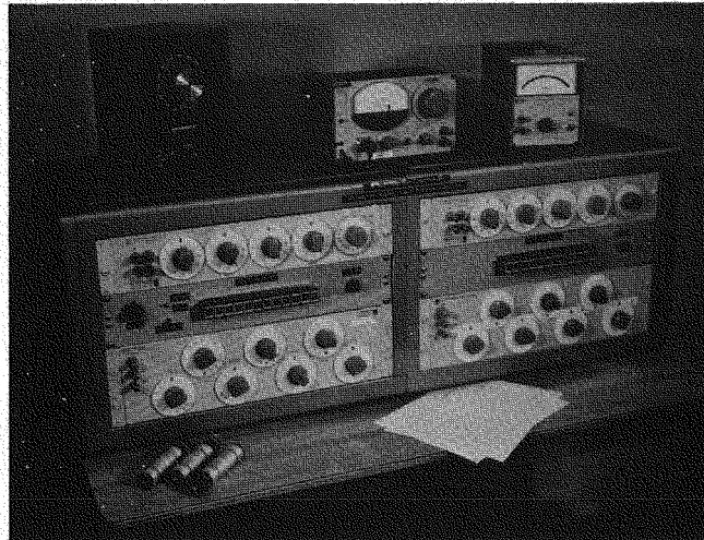
Figure 3-2. TESTING OF CABLES UTILIZING PRECISION A-C RESISTANCE- REACTANCE BRIDGE
