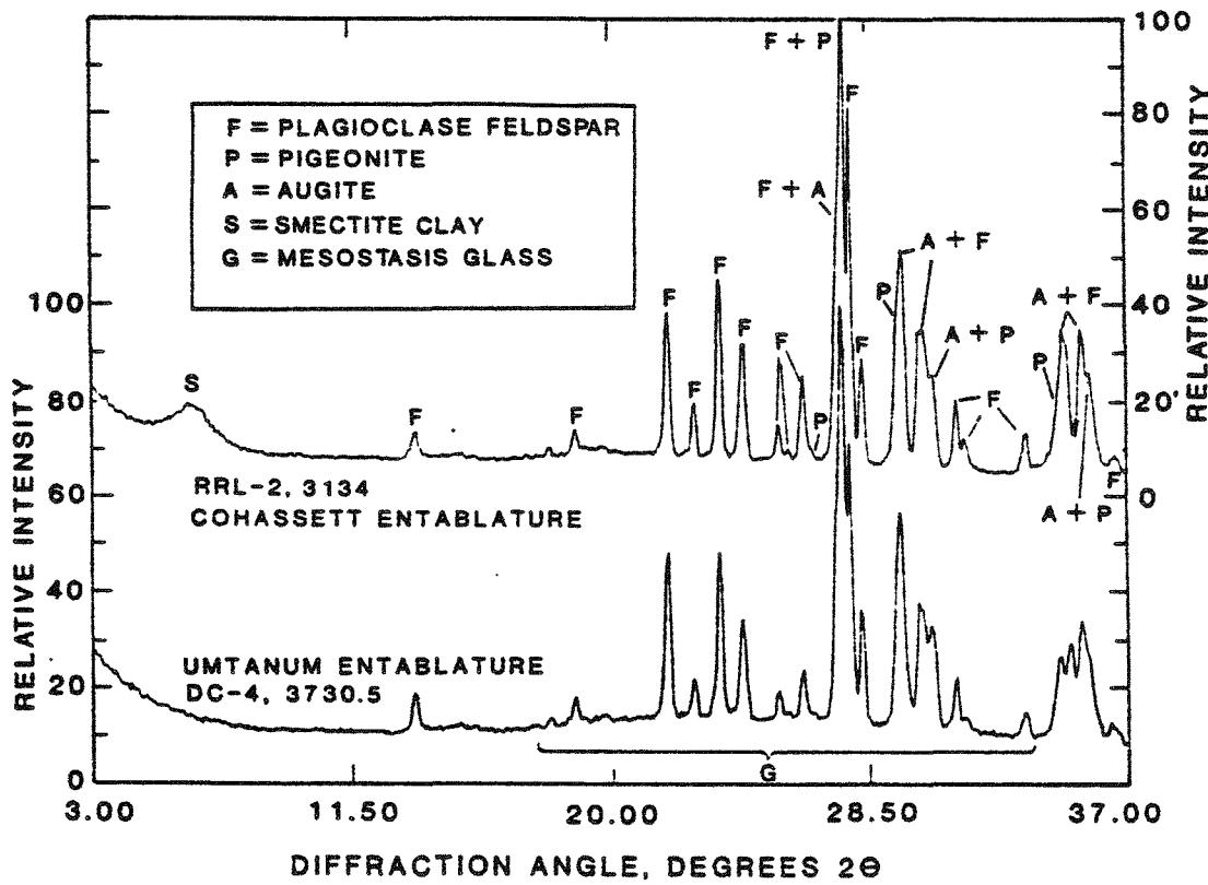
Figure 10. Comparison of X-ray diffractograms from core samples of the Cohassett and Umtanum entablature basalts. Minor differences in the primary mineral compositions are visible. No secondary clay is evident in the diffractogram of the Umtanum sample, and evidence of mesostasis glass is absent from the Cohassett pattern.
