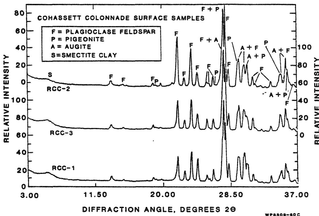
Figure 17. Comparison of X-ray diffractograms from three surface samples of reference Cohassett colonnade basalt. Differences among these patterns are indicative of the small compositional variations observed in this material by other methods.
