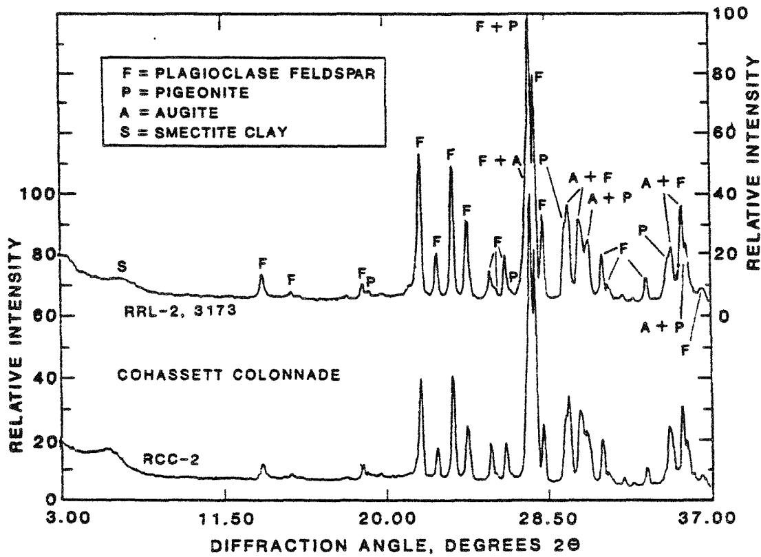
Figure 16. Comparison of X-ray diffractograms of Cohassett colonnade basalt from a core sample (RRL-2, 3173) and a surface sample (RCC-2). Only very minor differences are evident.
