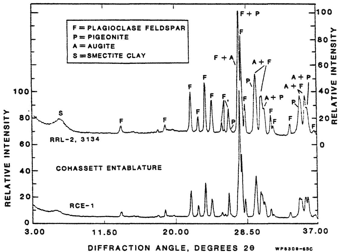
Figure 9. X-ray diffractograms of Cohassett entablature basalt from a core sample (RRL-2, 3134) and a surface sample (RCE-1).
