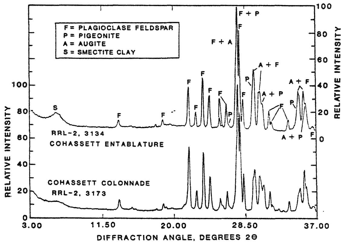
Figure 15. X-ray diffractograms of Cohassett entablature and colonnade samples from core hole RRL-2. Note the differences in the augite peaks, as well as in the intensities of the smectite clay peaks.
