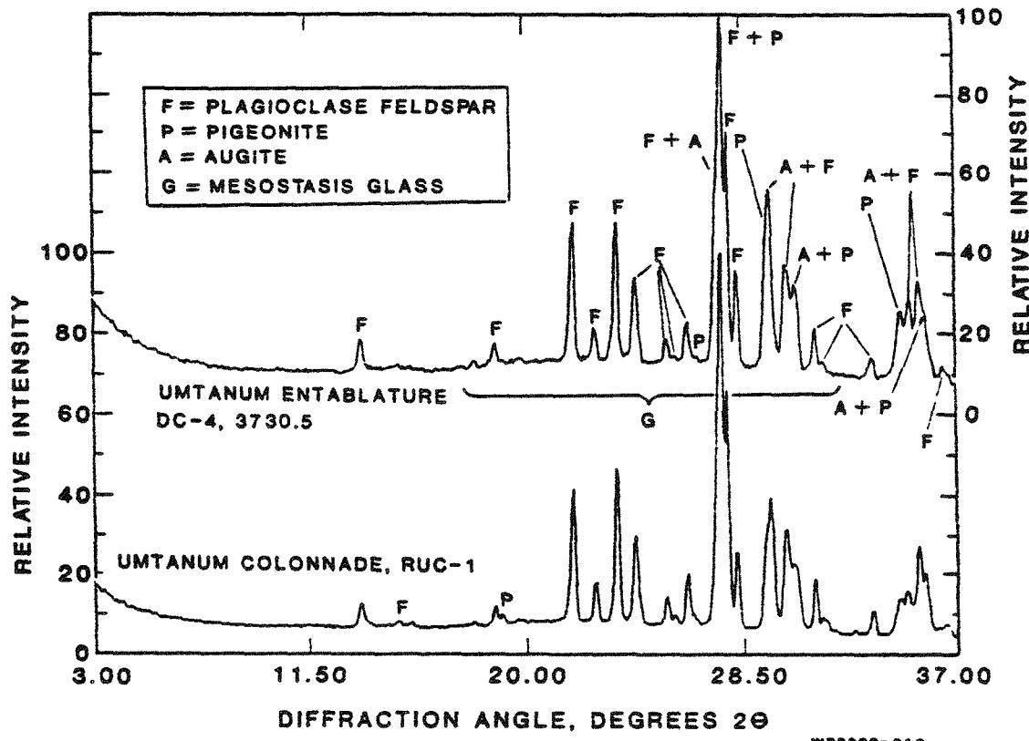
Figure 5. Comparison of X-ray diffractograms from the Umtanum entablature and colonnade.
