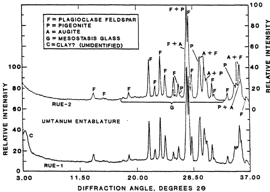
Figure 4. X-ray diffractograms of Umtanum entablature basalt from surface samples RUE-1 and RUE-2, both in -120 +230 mesh size fractions. The clay peak (C) observed in the RUE-1 specimen is consistent with the alteration products phase reported in point count results from other RUE-1 samples (Table 1).
