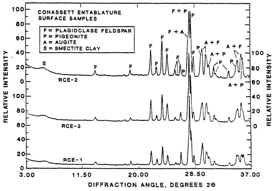
Figure 11. Comparison of X-ray diffractograms from three surface samples of reference Cohassett entablature basalt.
