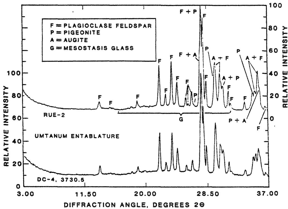
Figure 3. X-ray diffractograms of Umtanum entablature basalt from a surface sample (RUE-2) and a core sample (DC-4, 3730.5). All diffractograms were produced from randomly-oriented powder mounts, using copper  $K\alpha$  radiation.
