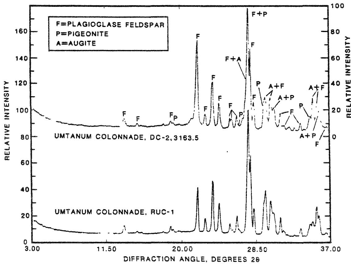
Figure 6. X-ray diffractograms of core (DC-2, 3163.5) and surface (RUC-1) samples of Umtanum colonnade.
