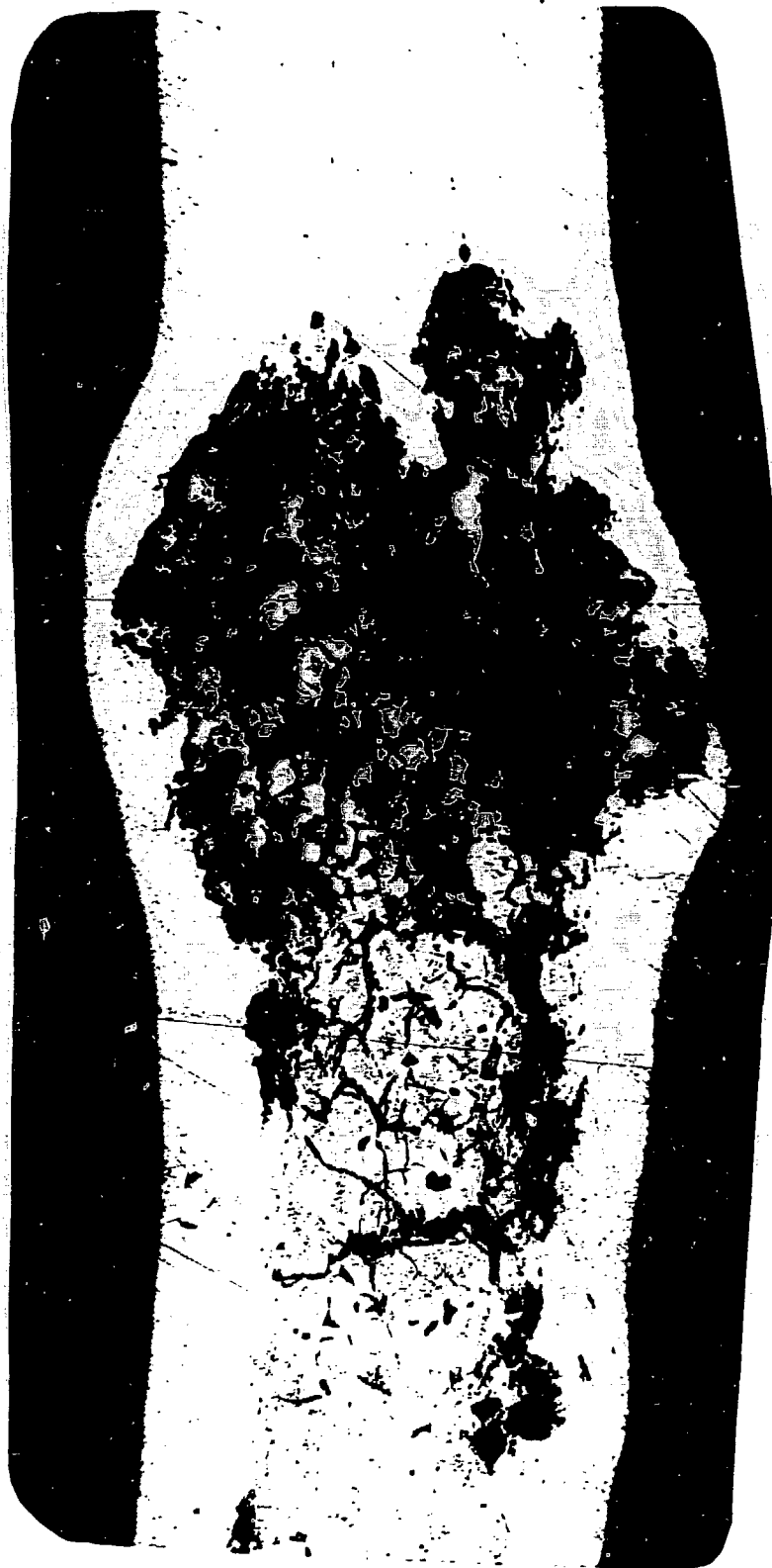
Fig. 7. Crosssection of Ruptured Blister at Dog Bone End of Irradiated \text{U}_3\text{Si}_2 Plate After Prolonged Annealing at 450°C
