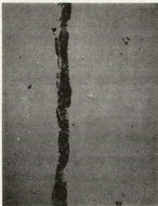
Figure 7. 100X Nomarski micrograph of line plated using single slow scan.
