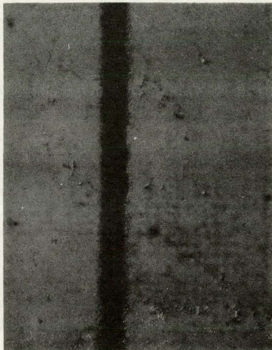
Figure 8. 200X Nomarski micrograph of line plated using multiple rapid scans.
