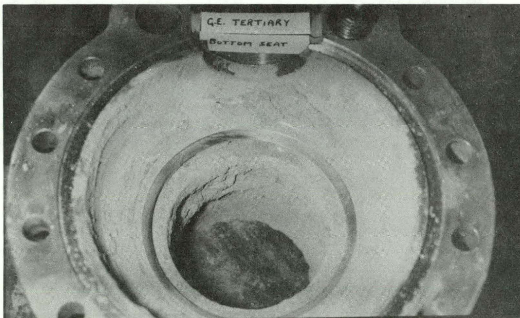
Fig.L60 Ball and lower scraper seat of Stream 2 tertiary dust system isolation valve after 1000 hrs.
