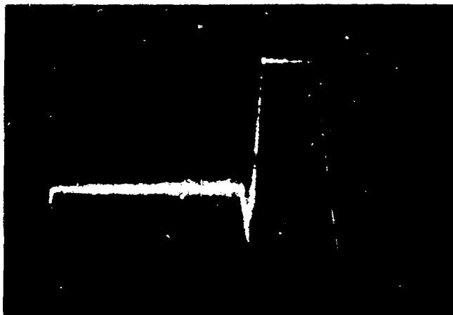
Fig. 5. Oscillogram of the pulsed voltage on the injection magnet chamber, using the circuit of fig. 6.
