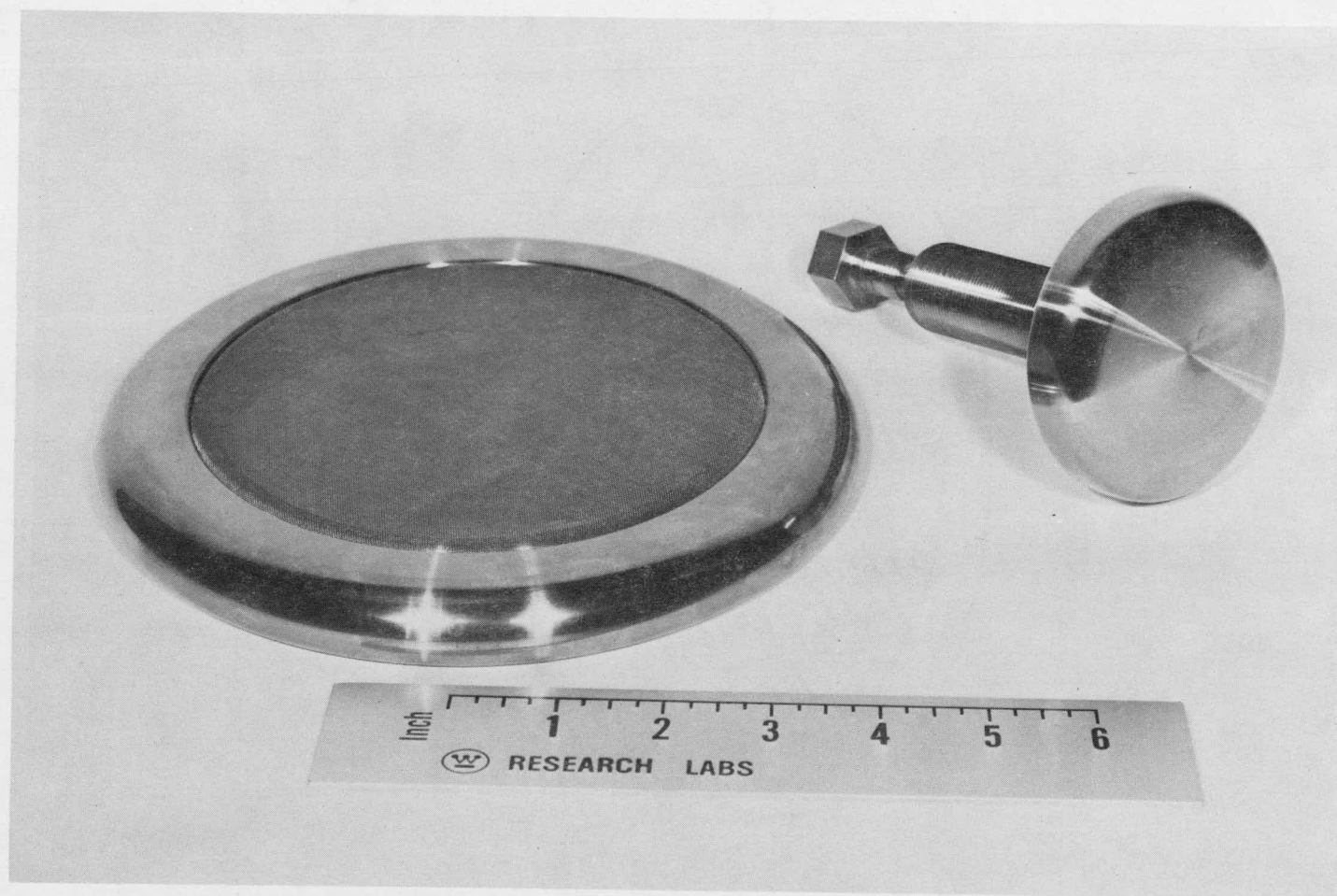
Fig. 11. Photograph of the anode (left) and cathode (right) used in the experimental studies.
