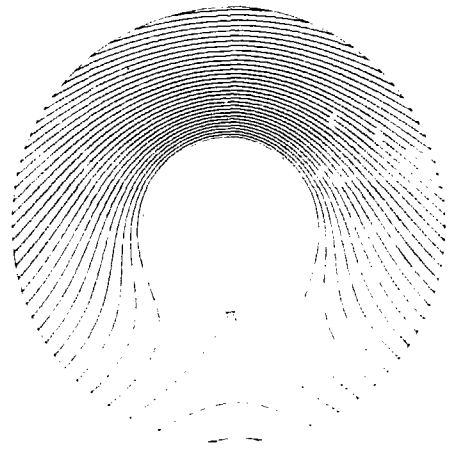
Fig. 6(a) - Uniform horizontal flow over a cylinder with circulation [ \Gamma/(RU) = 2 ].
