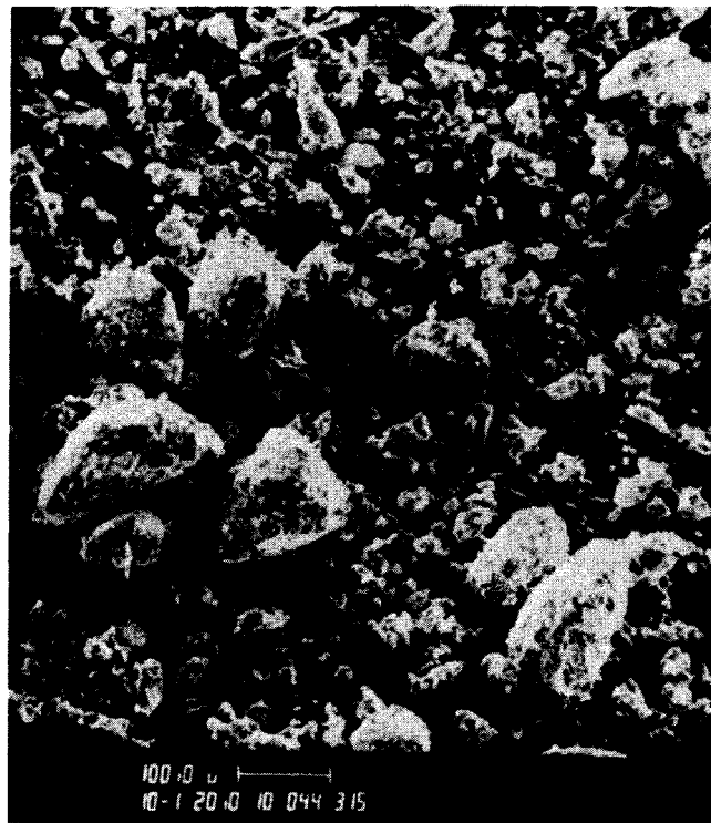
Figure 1.27. SEM PHOTOGRAPH OF AD55-2D AS-RECEIVED POWDER (100 X)
