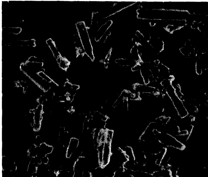
Figure 1.11. SEM MICROGRAPH OF \text{LiAlO}_2 PARTICLES WASHED FROM FINAL ELECTROLYTE AD55-1A (5000X)
