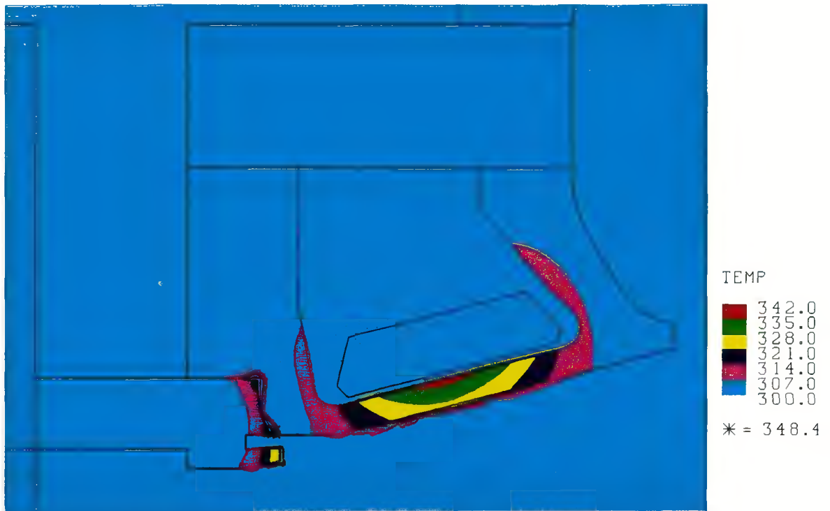
Figure 11: Temperature field in the diode at the peak of the current pulse.
