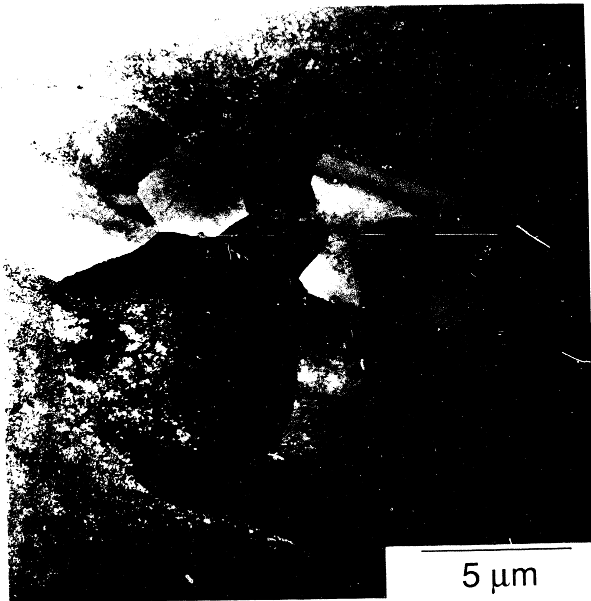
Figure 6: TEM micrograph of the grain structure at quarter-thickness. Note the inhomogeneous distribution of subgrains. Isolated grains composed of subgrains are found between large grains that do not contain subgrains. (XBB 915-4150)
