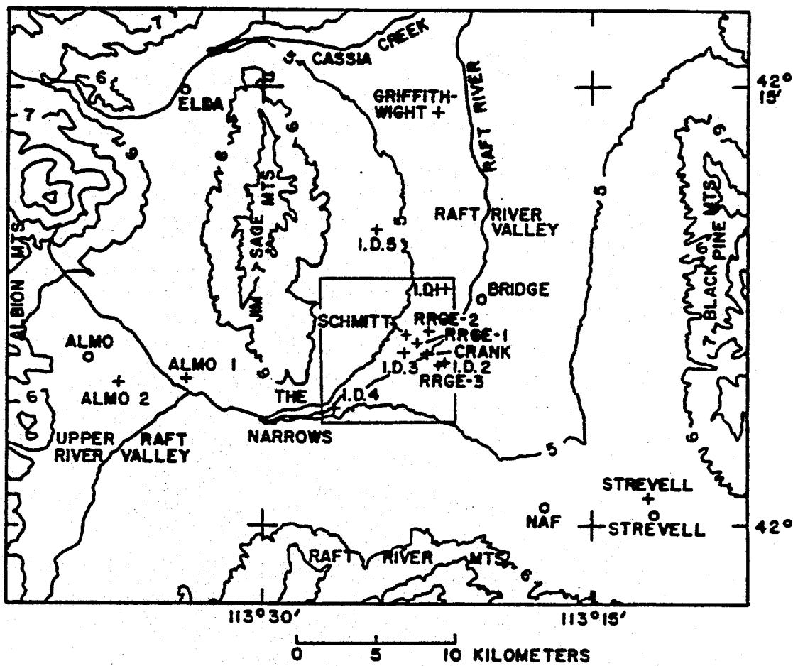
FIG. 1. Topographic map (1000-foot contours) of Raft River geothermal area and environs. Crosses, well and drill-hole locations; circles, towns. Area of Figure 5 is outlined.
