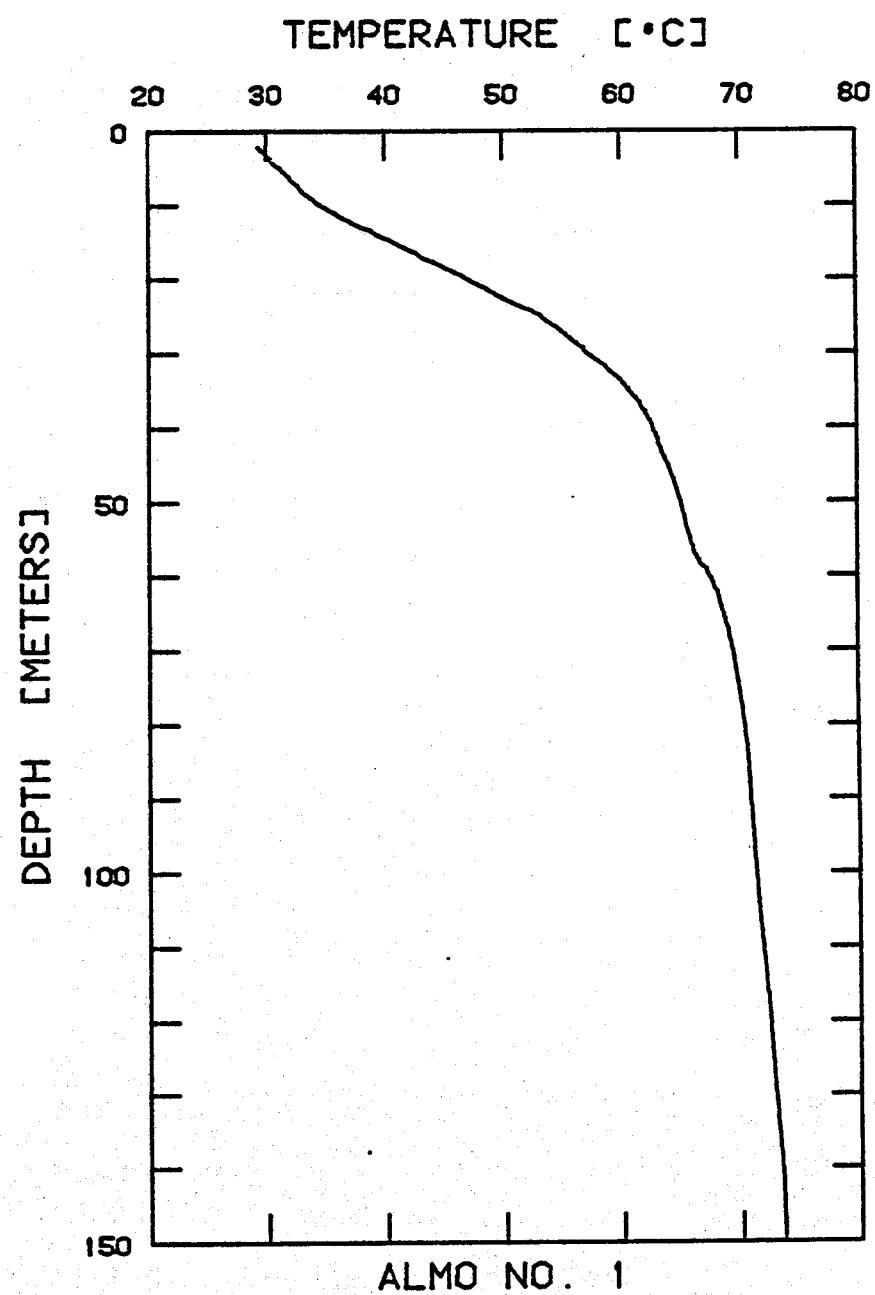
FIG. 10. Temperature log of drill hole Almo 1, obtained on 7 August 1976. Wellhead pressure of 0.79 bar gauge at 0.5 m above ground level. Flowing 3 mL/sec prior to logging.
