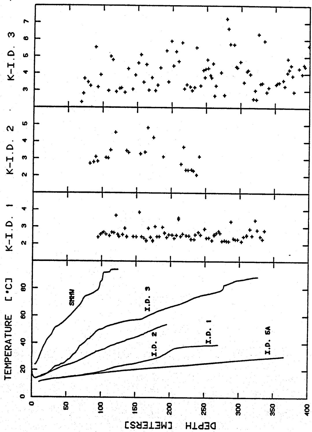
FIG. 8. Temperature logs of drill holes I.D. 1, 2, 3, and 5A, and SMHW; see Figures 1 and 5 for locations. Temperatures measured on 15 January 1976 (I.D. 1, 2), 6 August 1976 (I.D. 5A), 11 August 1976 (I.D. 3), and 14 August 1976 (SMHW). Wellhead pressure of 0.9 bar gauge at ground level in I.D. 3 during logging with no flow. Thermal conductivities are in  $\text{mcal/cm sec } ^\circ\text{C}$ .
