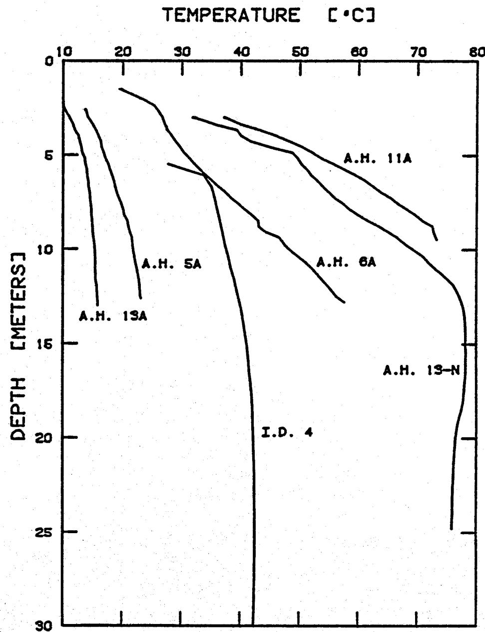
FIG. 6. Temperature logs of group I auger holes, I.D. 4, and A.H. 13A; see Figure 5 for locations. Temperatures measured on 16 January 1976 (A.H. 11A), 17 January 1976 (A.H. 13A, 13-N), 9 February 1976 (A.H. 5A), 8 August 1976 (I.D. 4), and 16 August 1976 (A.H. 6A).
