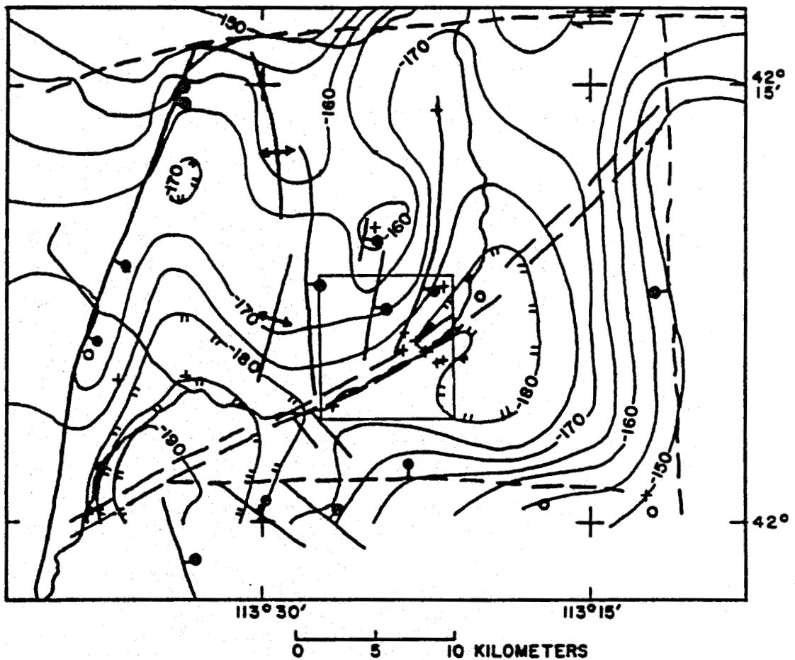
FIG. 2. Map of Bouguer anomaly values calculated with a  $2.67\text{-g/cm}^3$  density factor (Mabey and Wilson, 1973); contour interval, 5 mGal (1 Gal =  $1\text{ cm/sec}^2$ ). Areas of low gravity are shown with hatched contours. Major faults (bar and ball on downthrown side—dashed where inferred) and anticline (Jim Sage Mountains only) from Williams et al (1976). Crosses, wells; circles, towns. Area of Figure 5 is outlined.
