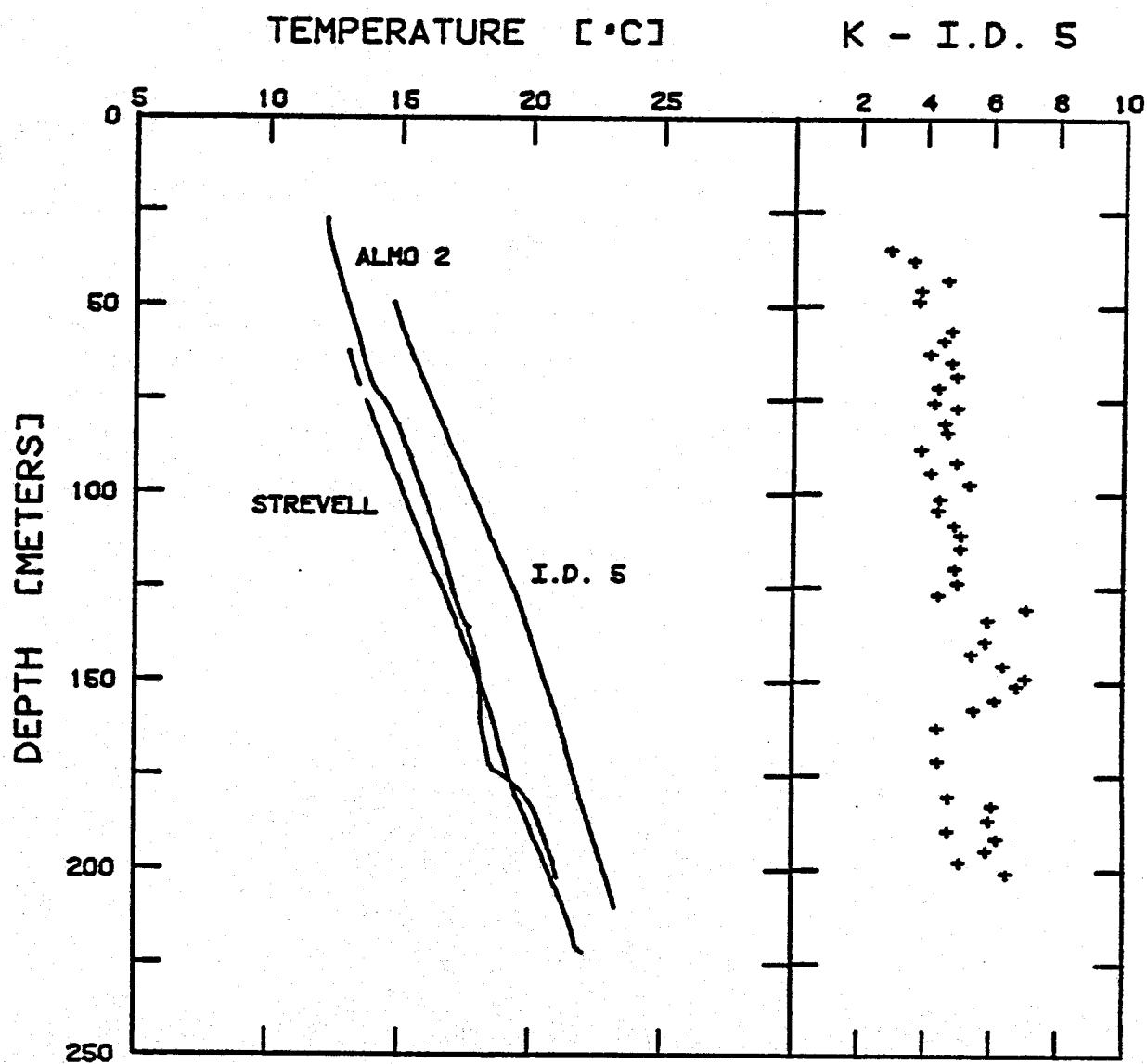
FIG. 3. Temperature logs in drill holes Strevell (17 October 1975), I.D. 5 (6 August 1976), and Almo 2 (8 August 1976). Strevell cased to logged depth, I.D. 5 cased and cemented to total depth, and Almo 2 cased to 141 m but cemented only to 70 m. Thermal conductivities for I.D. 5 are in  $\text{mcal}/\text{cm sec } ^\circ\text{C}$ .
