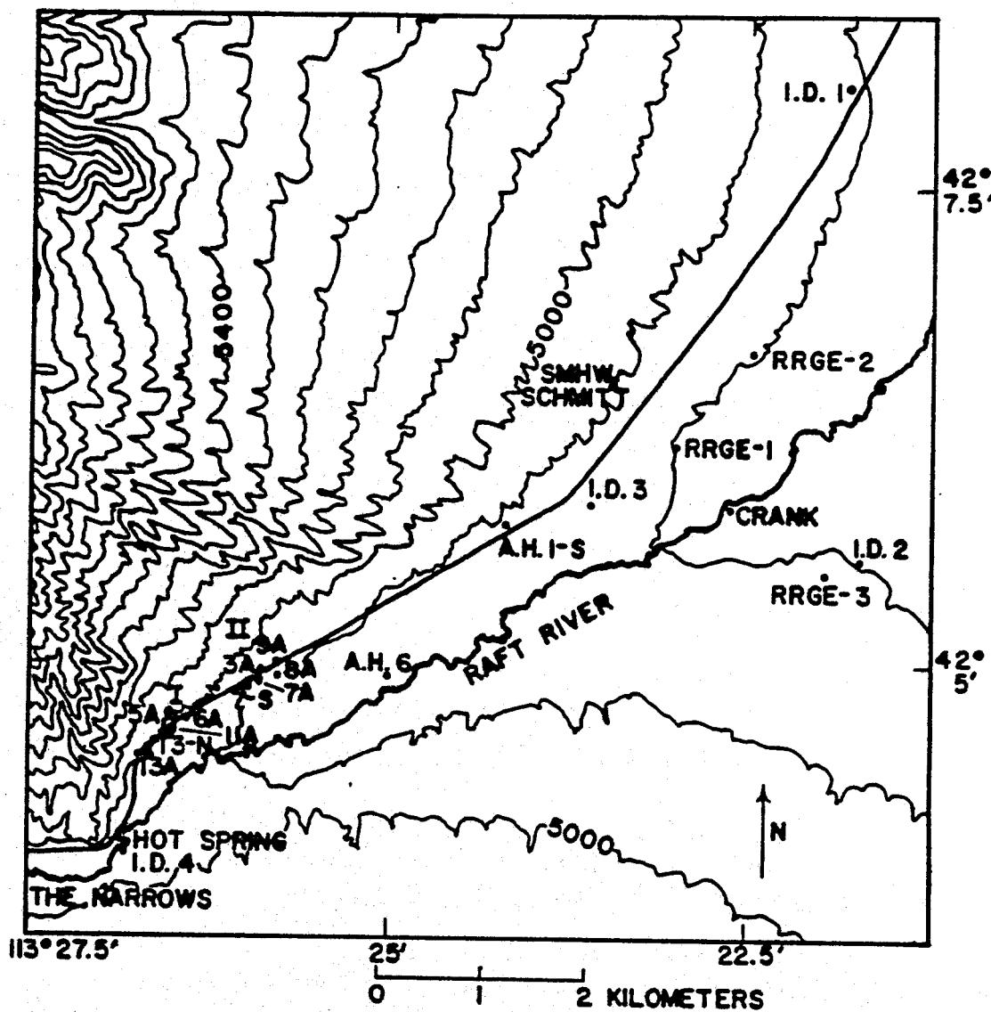
FIG. 5. Topographic map (80-foot contour interval) showing locations of auger holes (A.H.), intermediate-depth drill holes (I.D.), Raft River geothermal exploration wells (RRGE), drill hole SMHW, and Schmitt and Crank hot wells. I and II denote groups of auger holes. See Figures 1 and 2 for general location of map.
