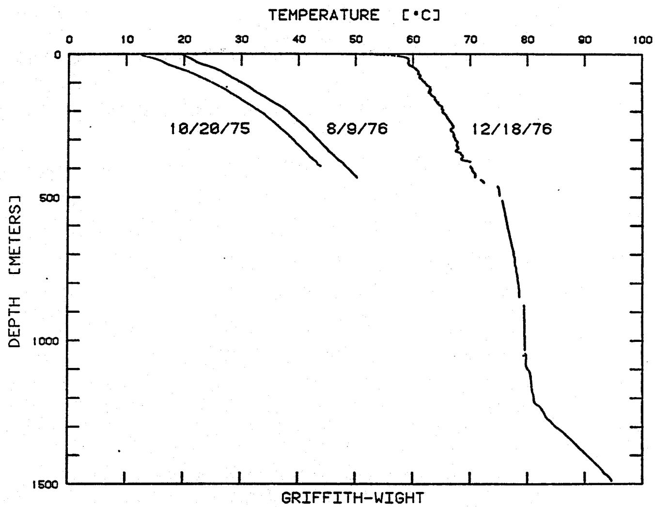
FIG. 4. Temperature logs in Griffith-Wight well. Log of 20 October 1975 was taken with no flow. Log of 9 August 1976 taken after well had been flowing 10 mL/sec for some time. Log of 18 December 1976 taken while intermittently flowing the well to get past zones where the temperature probe stuck.
