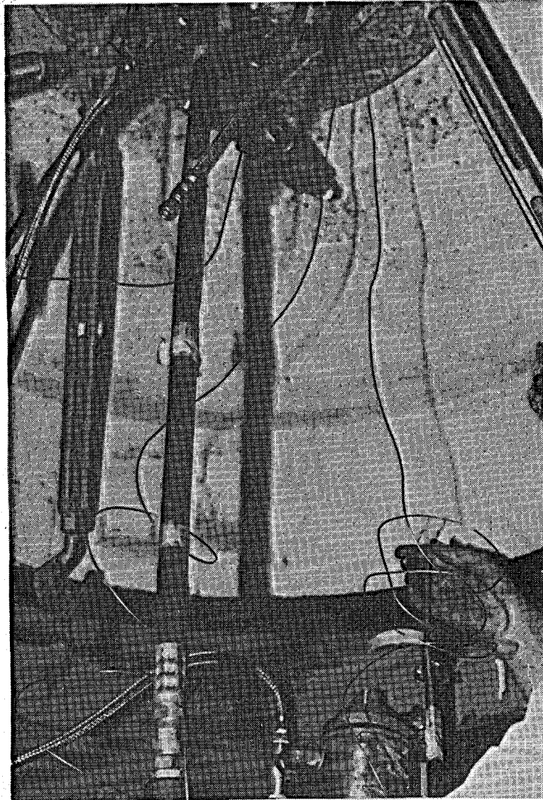
Figure 5. Thermocouple wires inside the lid of the 48-inch diameter pressure vessel prior to test. Tube (at hand in photo) is exit passage of foam to which canvas bag was attached.
