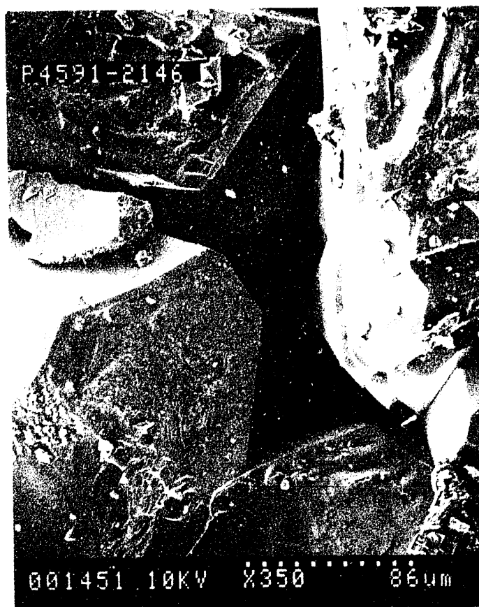
Figure 49.--Secondary-electron micrograph of a pore and pore throat surrounded by quartz overgrowths on detrital quartz grains (Carter sandstone, Wayside oil unit, well PN4591, 2,146 ft., scale is on photograph).
