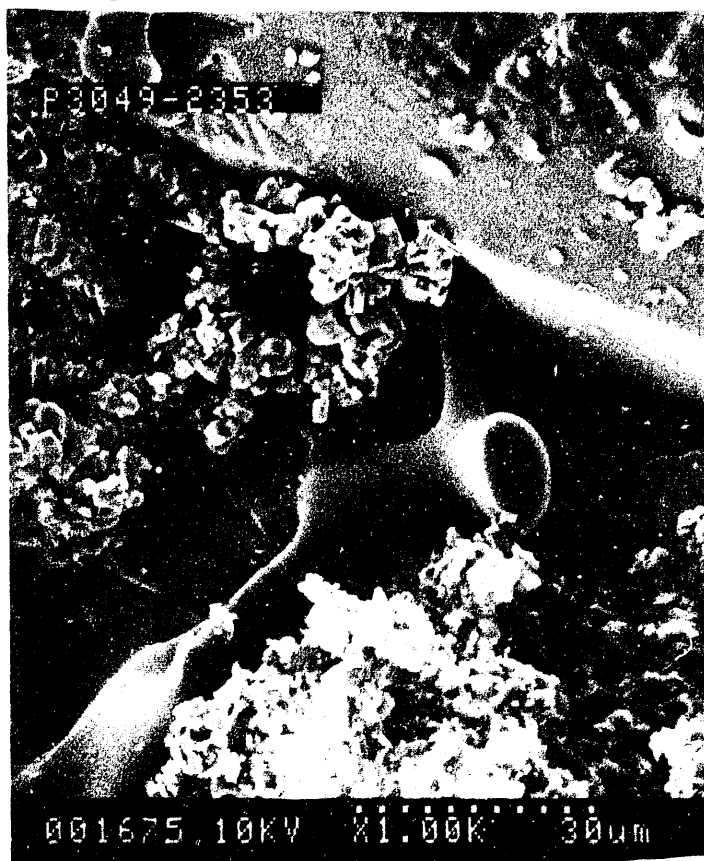
Figure 61.--Secondary-electron micrograph of hydrocarbon residue (Carter sandstone, North Blowhorn Creek oil unit, well PN3049, 2,353 ft; scale is on photograph). The hydrocarbon residue is the cylindrical object in the center of the photograph. The residue is attached to a quartz overgrowth. Note authigenic kaolinite in upper left half of photograph.
