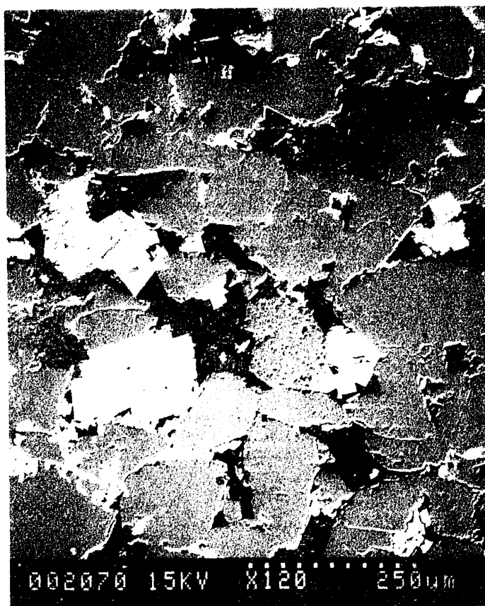
Figure 67.--Backscattered-electron micrograph of pore system in Carter sandstone (Carter sandstone, North Blowhorn Creek oil unit, well PN3160, 2,303.4 ft; scale is on photograph). Pores are black. Note intergranular pores and microporosity within kaolinite (center) and partially dissolved intrabasinal shale fragments (upper right). Light gray crystals are ferroan dolomite/ankerite.
