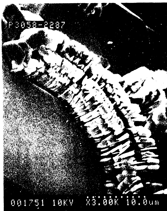
Figure 54 --Secondary-electron micrograph of a single stack of authigenic "kopy-kat" kaolinite (Carter sandstone, North Blowhorn Creek oil unit, well PN3058, 2,287 ft; scale is on photograph). Note the groove that extends the length of the stack. The kaolinite is partially encased by a quartz overgrowth.
