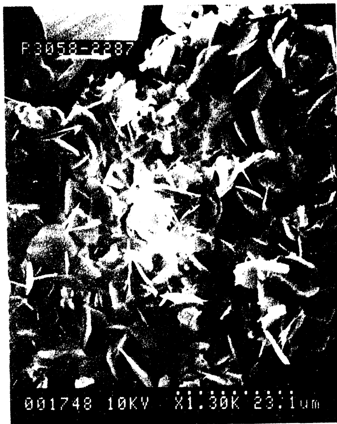
Figure 36 --Secondary-electron micrograph of face-to-face and face-to-edge flakes of chlorite in an intrabasinal mud fragment (Carter sandstone, North Blowhorn Creek oil unit, well PN3058, 2,287 ft, scale is on photograph).
