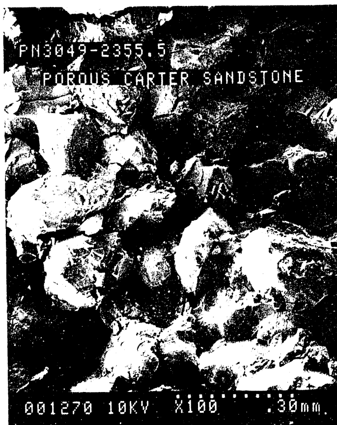
Figure 64--Secondary-electron micrograph of the pore network in Carter reservoir sandstone (Carter sandstone, North Blowhorn Creek oil unit, well PN3049, 2,355.5 ft, scale is on photograph). The fractured material in some pores is hydrocarbon residue.
