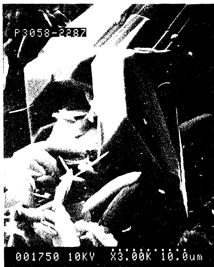
Figure 58.--Secondary-electron micrograph of authigenic quartz crystals partially enclosing plates of authigenic chlorite (Carter sandstone, North Blowhorn Creek oil unit, well PN3058, 2,287 ft; scale is on photograph). This relationship shows that chlorite formed prior to quartz.
