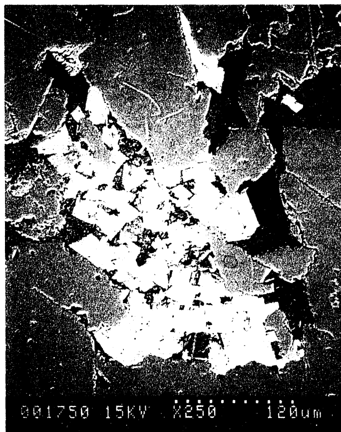
Figure 45.--Backscattered-electron micrograph showing ferroan dolomite/ankerite replacement of an intra-basinal mud clast (Carter sandstone, North Blowhorn Creek oil unit, well PN3160, 2,311.7 ft; scale is on photograph). Light gray areas are ferroan dolomite/ankerite, medium gray grains are quartz, and black areas are pores.
