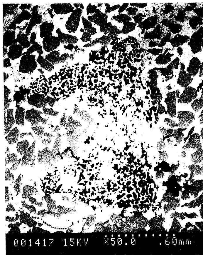
Figure 65.--Backscattered-electron micrograph of partially dissolved fossil fragments in pervasively calcite and ferroan dolomite/ankerite cemented sandstone (Carter sandstone North Blowhorn Creek oil unit, well PN3160, 2,302.5 ft; scale is on photograph).
