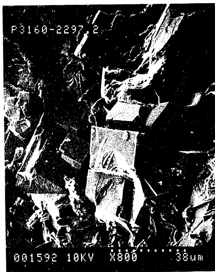
Figure 44.-Secondary-electron micrograph of a cluster of rhombic, authigenic ferroan dolomite/ankerite crystals (Carter sandstone, North Blowhorn Creek oil unit, well PN3160, 2,297.3 ft, scale is on photograph).
