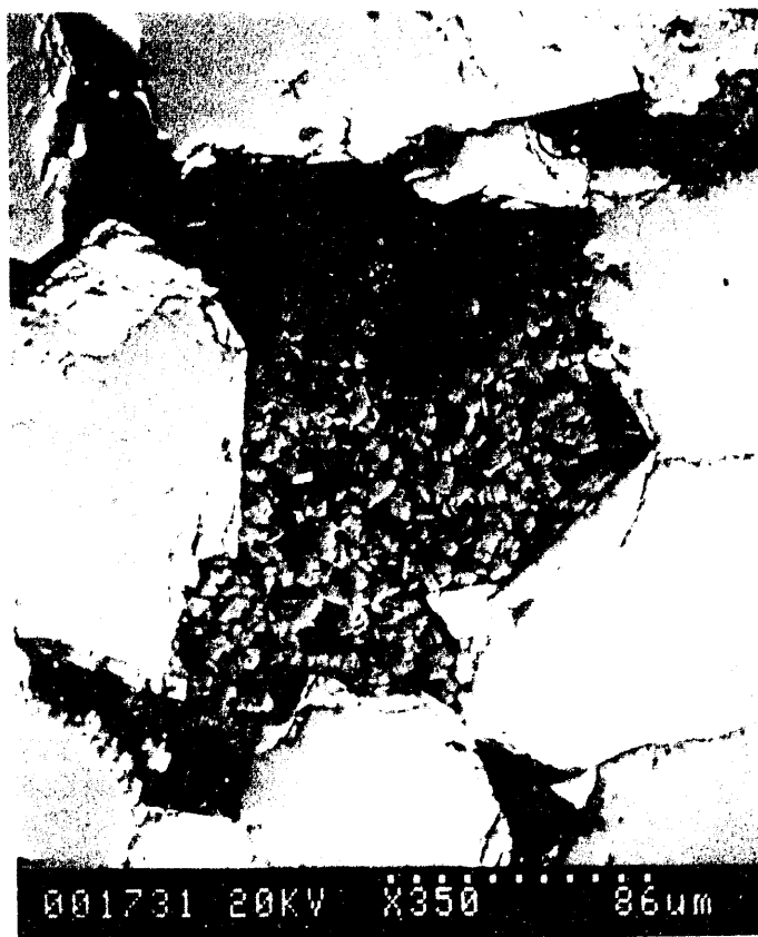
Figure 51 --Backscattered-electron micrograph of authigenic kaolinite partially filling a detrital grain size area and intergranular pores (Carter sandstone, North Blowhorn Creek oil unit, well PN3160, 3,211.7 ft; scale is on photograph).
