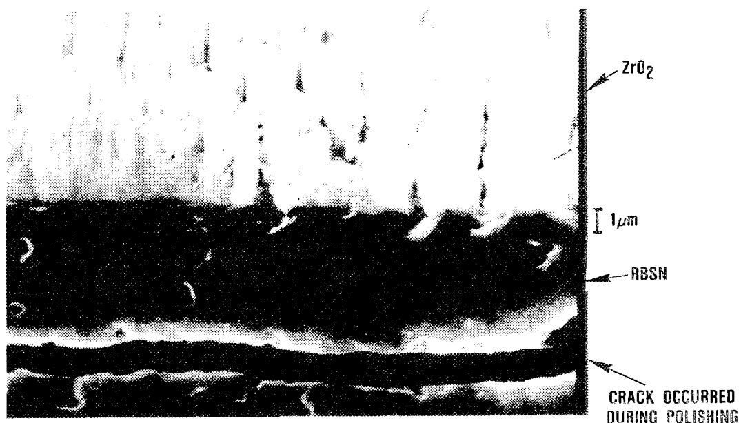
AS-COATED RBSN SILICATE LAYER NOT VISIBLE
