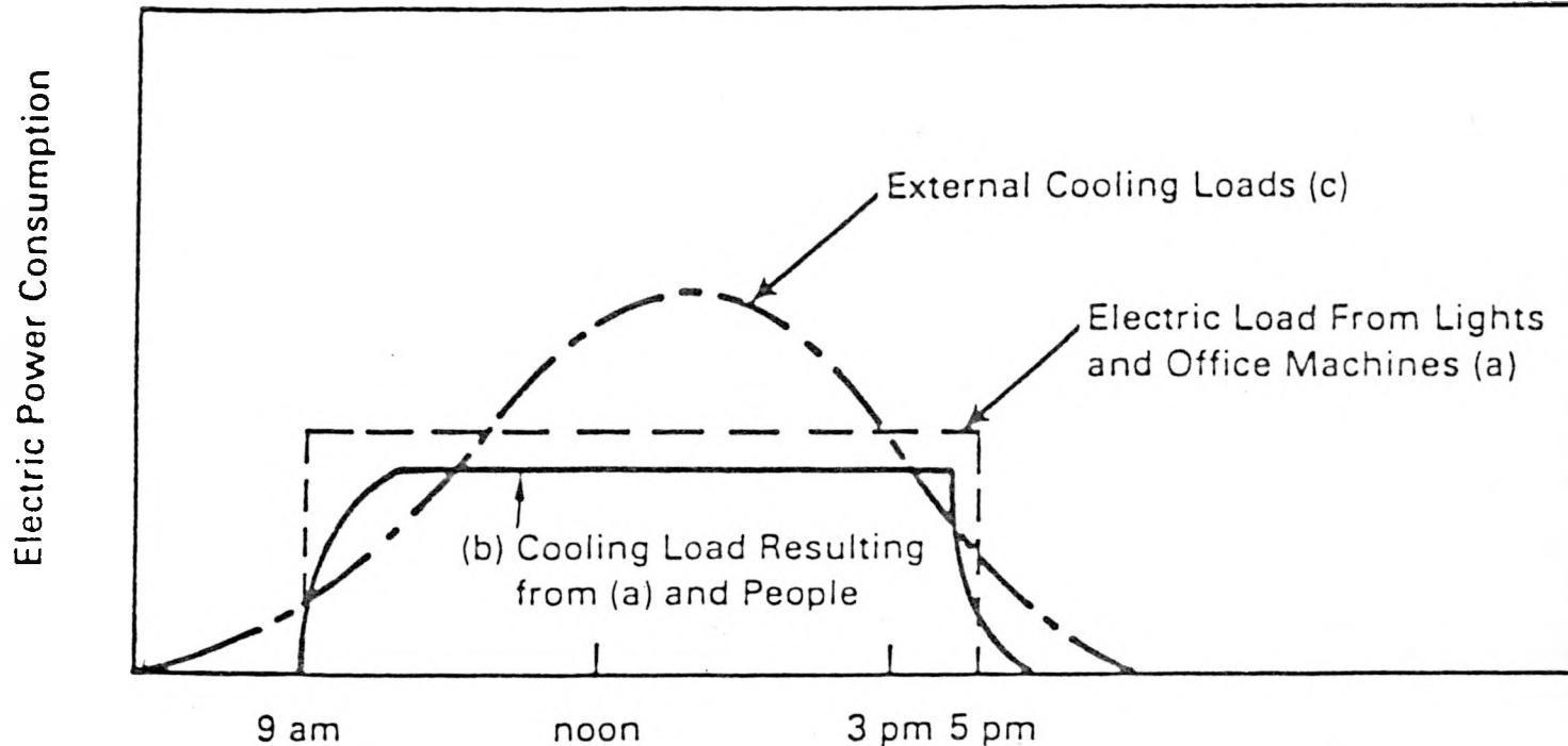
(B) Reduction of electrical loads as a result of daylighting
