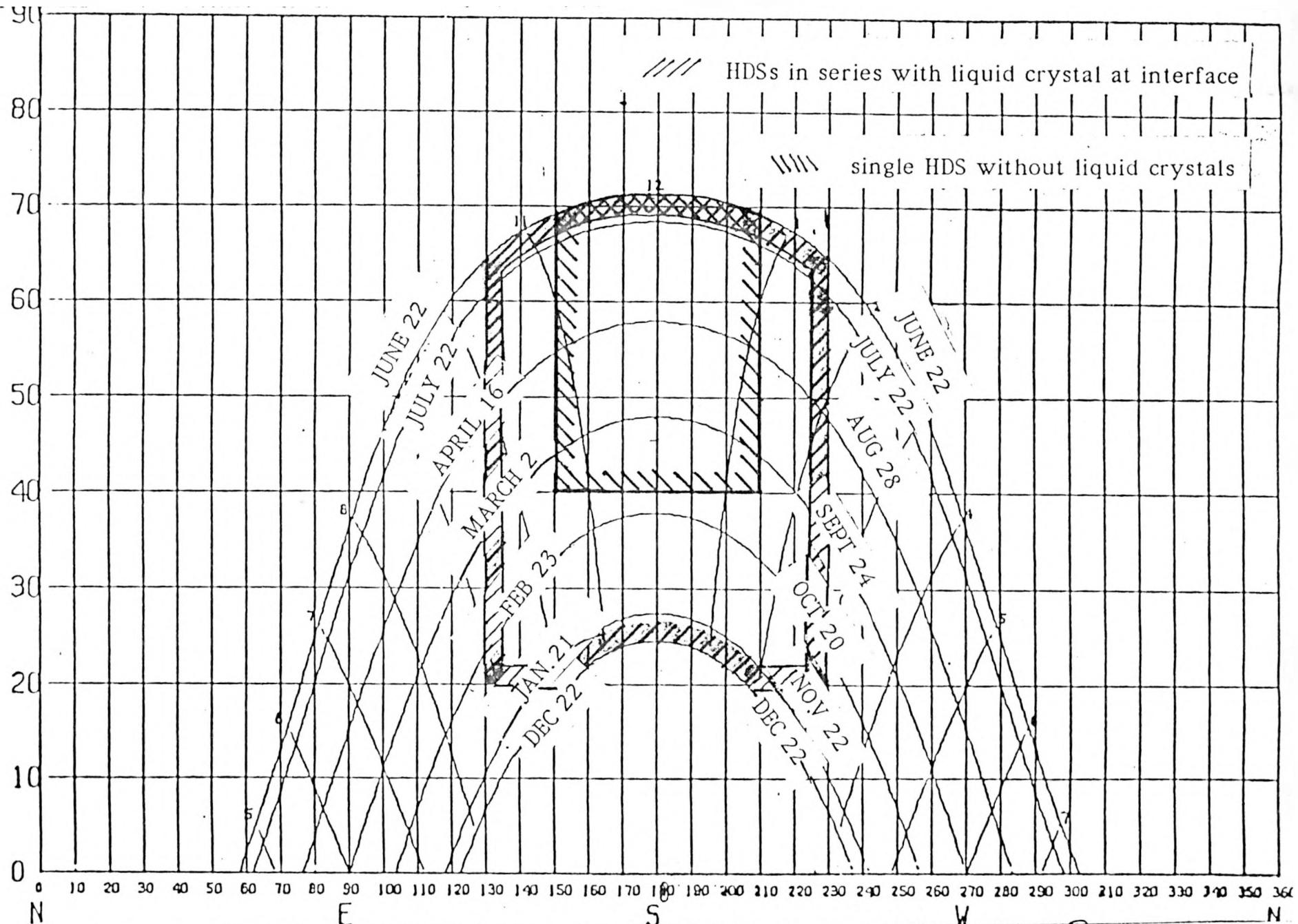
portion of the "sunpath" which could be passively "tracked" by the liquid-crystal filled holographic diffractive elements (theoretically).
