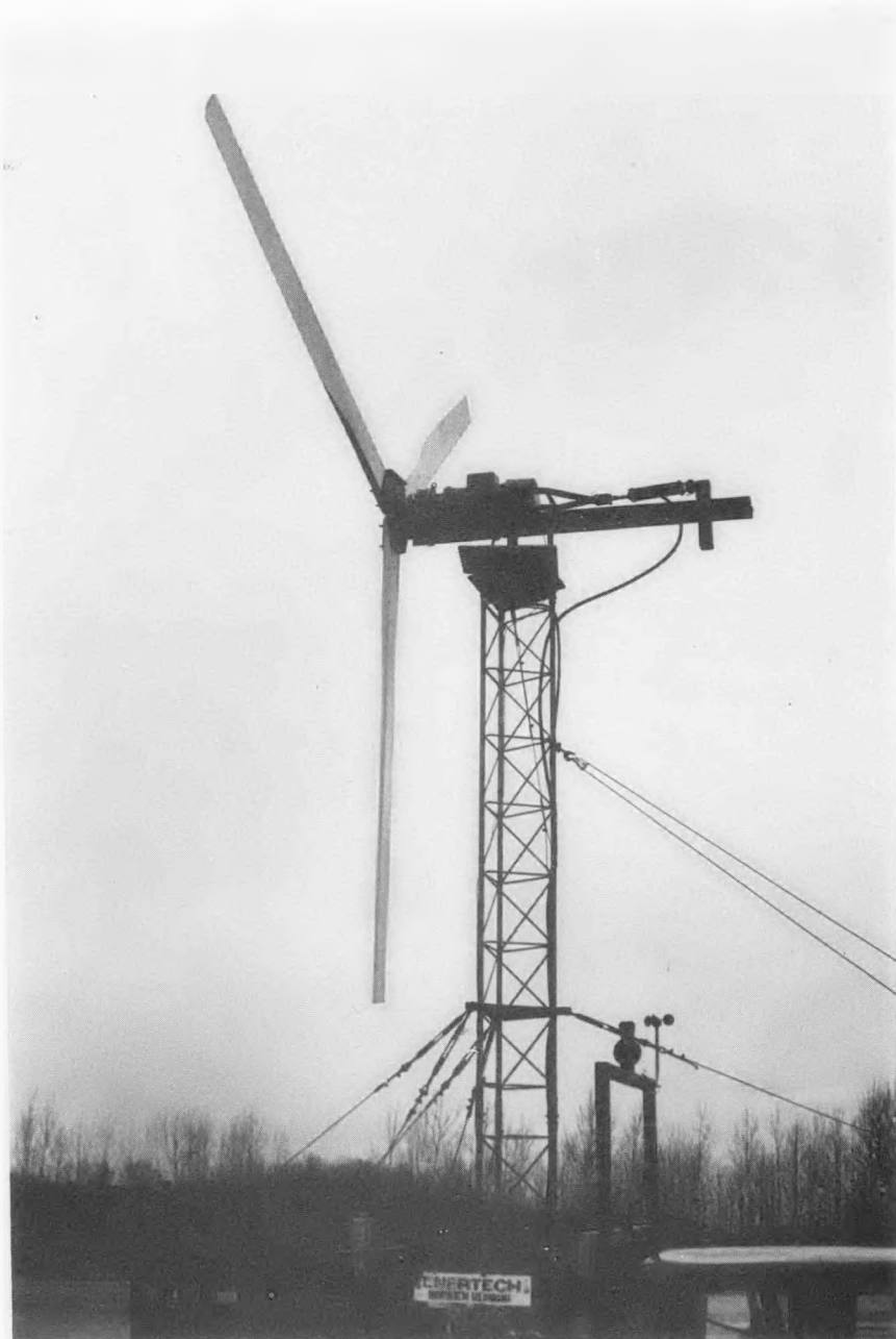
Figure 44 Thrust Test Set-Up on Test Truck
