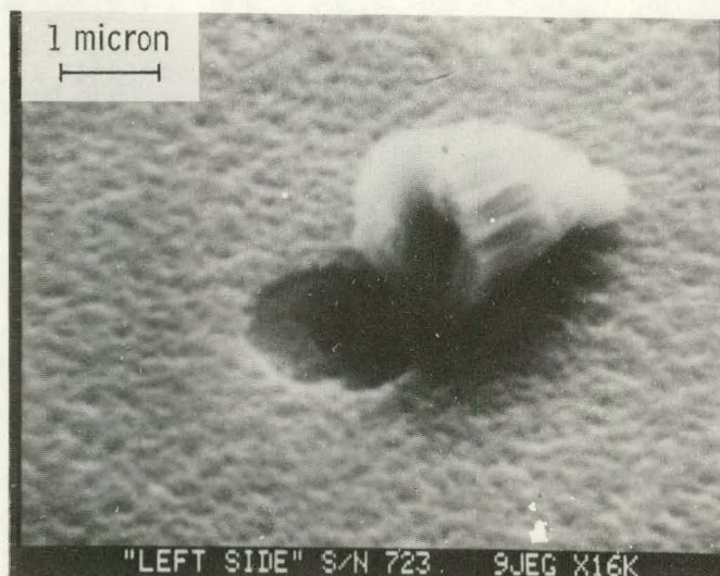
Fig. 11 Scanning electron microscopy photomicrographs showing copper nodules that form under certain conditions during \text{Cu}_x\text{S} deposition.
