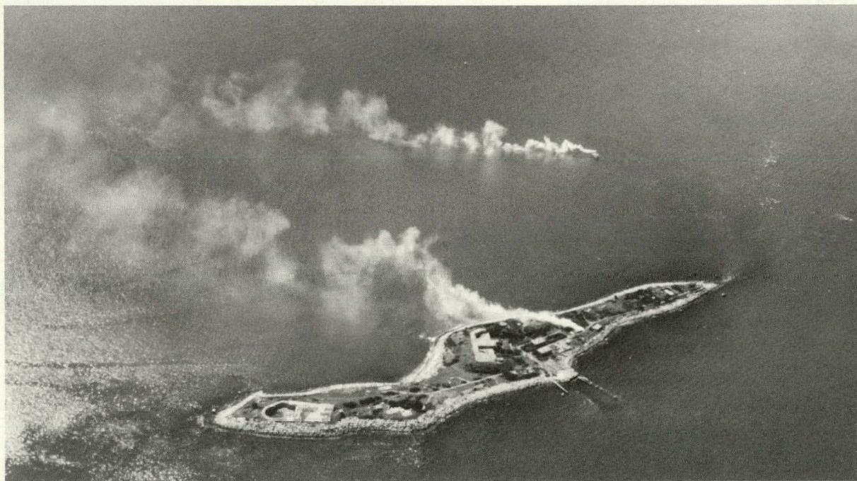
Figure 3. Smoke from generators is used to trace wind patterns. Here the behavior of winds in the wake of an island is being delineated by two plumes, one from the island and one from a ship anchored nearby.
