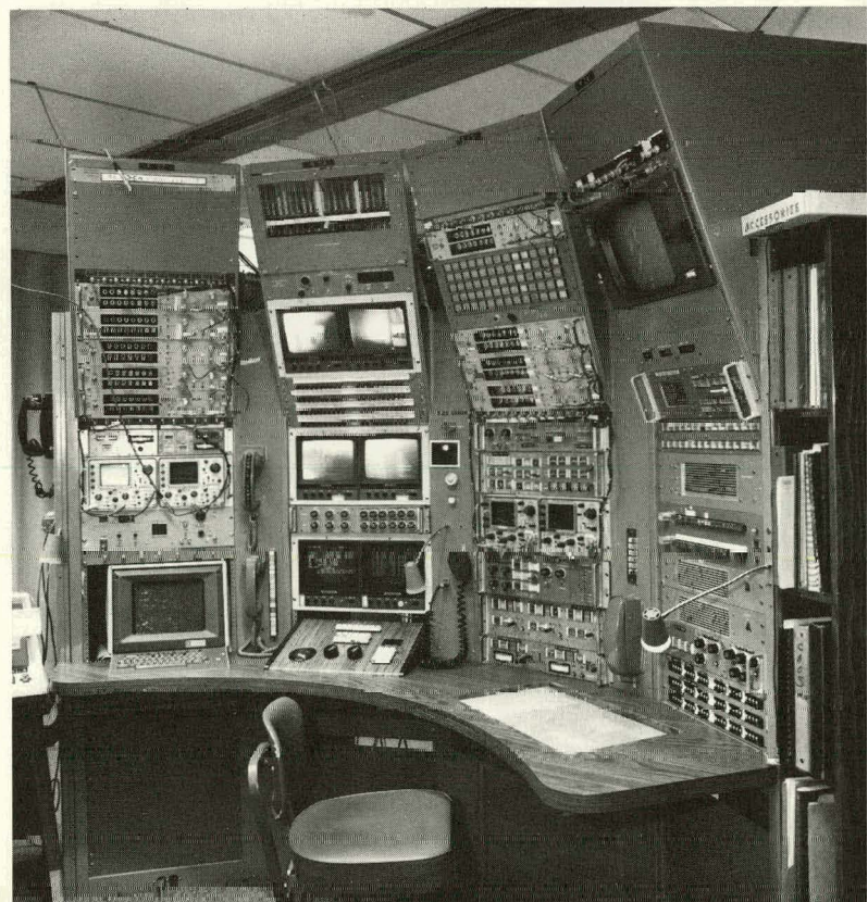
Figure 14. New external beam console in AGS Main Control Room which combines the control functions for both slow and fast external beams.
