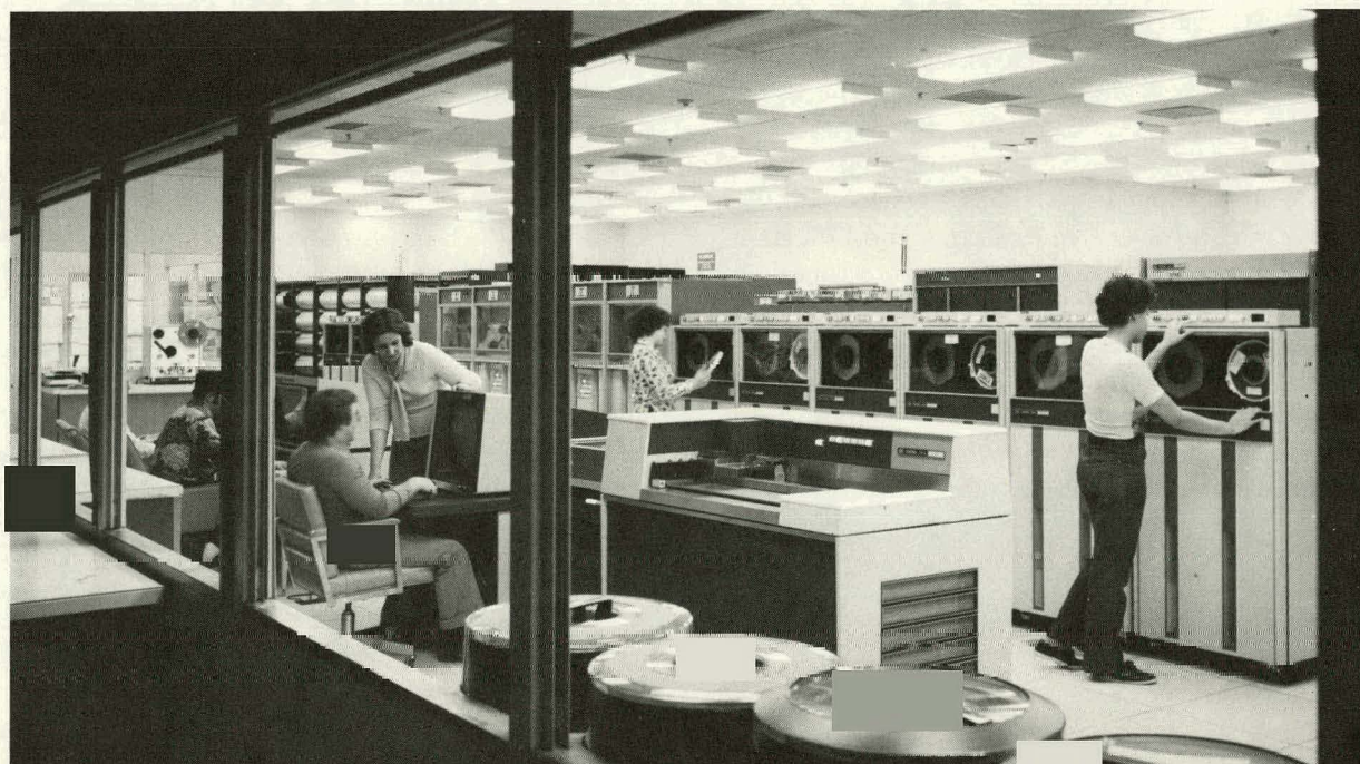
Figure 2. A view into the control console area of the CSCF from which computer operators interact with the CDC Cyber 70/76 and the two CDC 6600 computers. In the background, operators are mounting tapes containing data to be used in computations.
