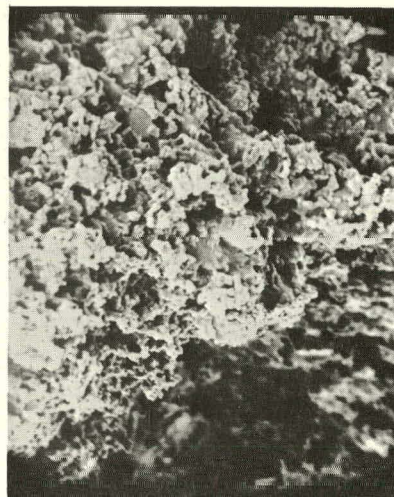
5401 + 5 mol % \text{CaCl}_2 Calcined 1h 850°C 1276X
