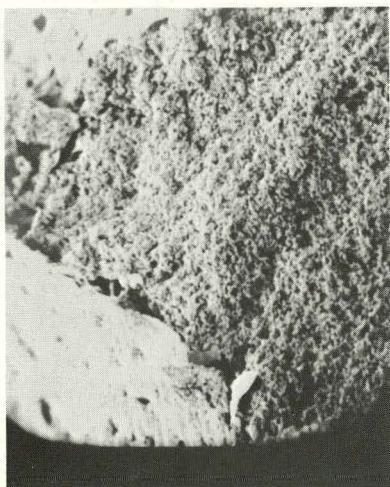
5601 + 0.5 mol % \text{CaCl}_2 Calcined 1h 850°C 638X
