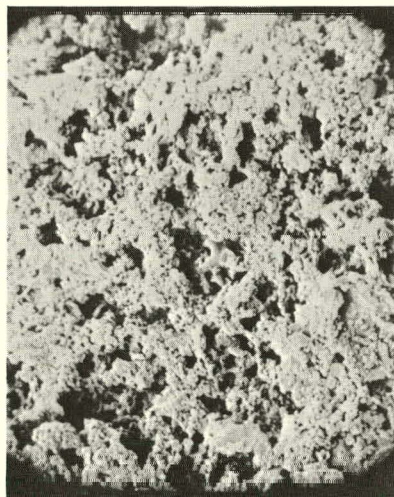
5401 + 3 mol % \text{CaCl}_2 Calcined 1h 850°C 1276X
