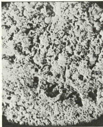
5601 + 1.0 mol % \text{CaCl}_2 Calcined 1h 850°C 638X
