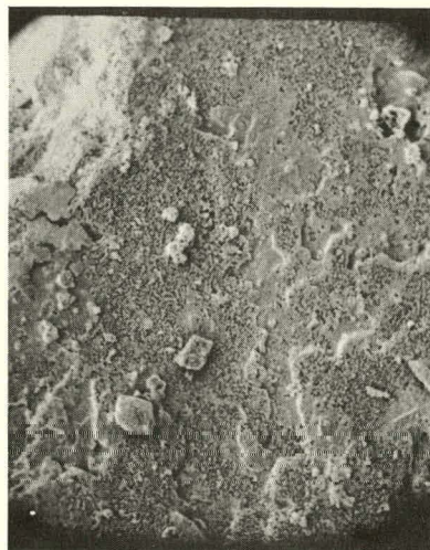
5401 + 0.1 mol % \text{CaCl}_2 Calcined 1h 850°C 1276X
