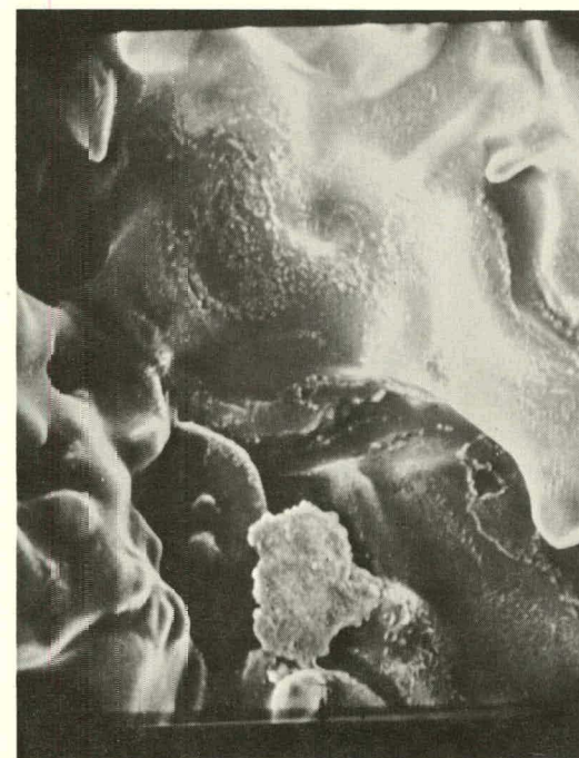
(c) 9501 + 2.0% \text{CaCl}_2 Junction of Two Particles 1920X
