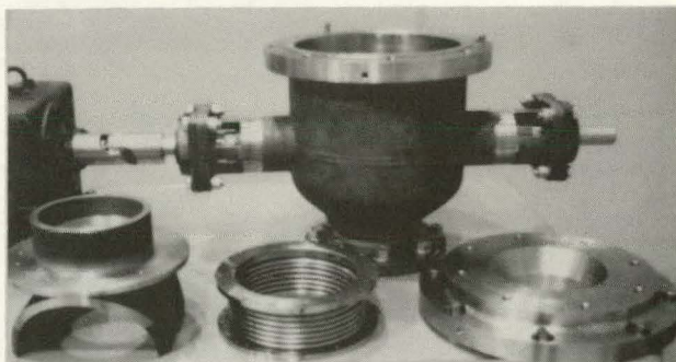
Fig. 3 High temperature rotary solids feeder rated for 700°C (1300°F) operation.
