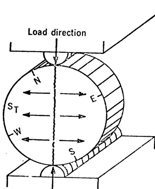
1. Each sample was broken in one of six directions,  $30^\circ$  apart. For example, one sample was broken at  $N60^\circ W$ , one at  $N30^\circ W$ , and one at  $N0^\circ$ . The remaining samples were broken at  $N30^\circ E$ ,  $N60^\circ E$ , and  $N90^\circ E$ , respectively.
