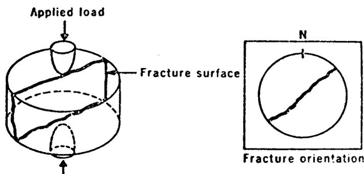
Fracture direction at random unless a "preferred direction" of failure exists.
