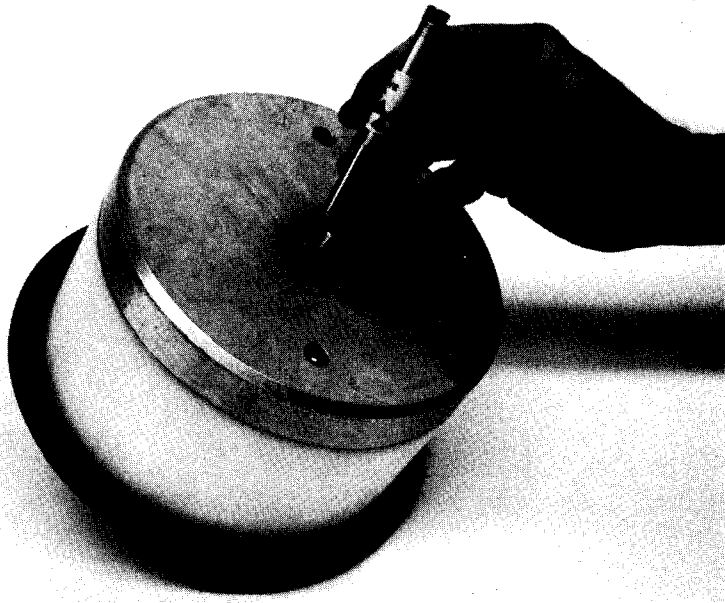
Fig. 14. The californium neutron source is stored in the top reflector cap of the HLNCC.
