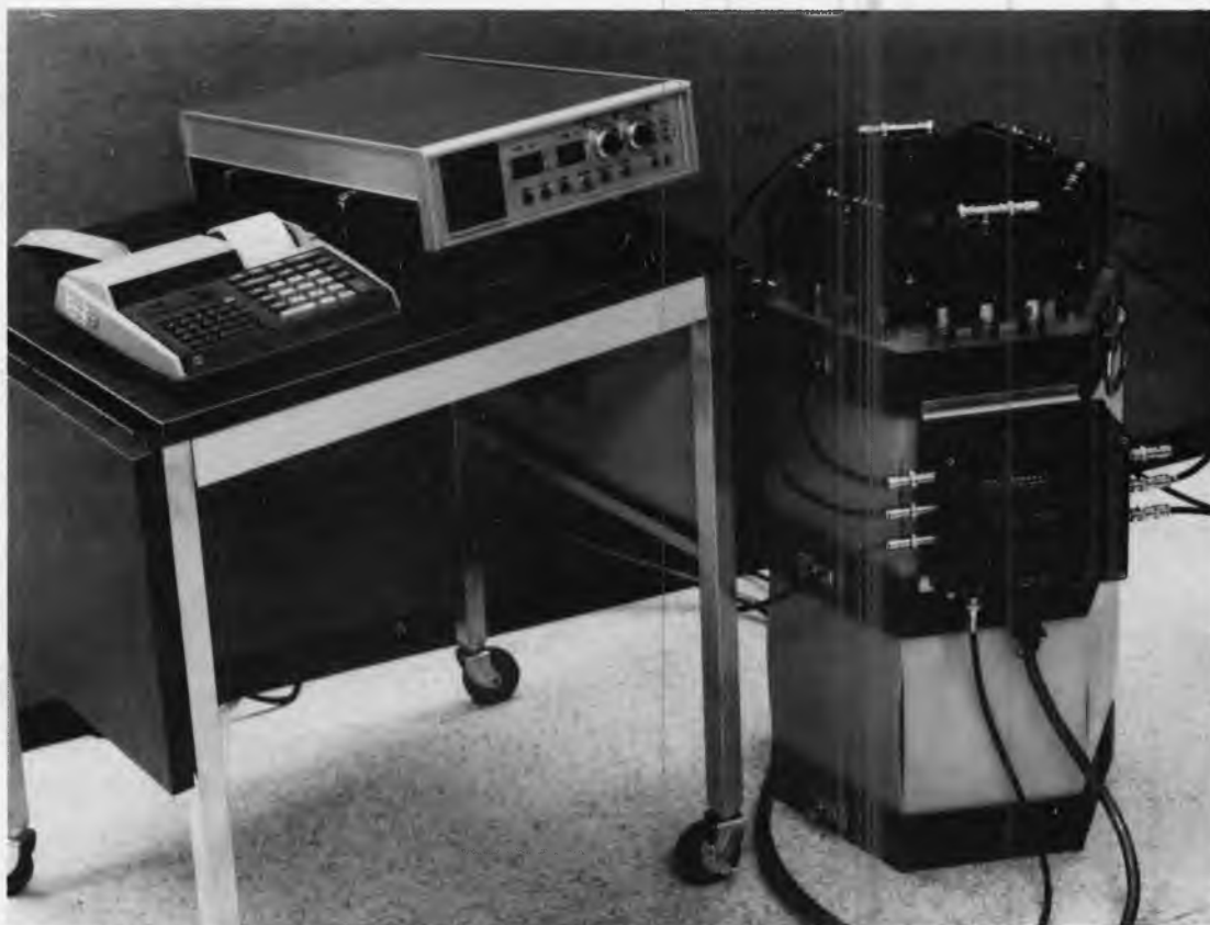
Fig. 1. HLNCC for plutonium assay.
