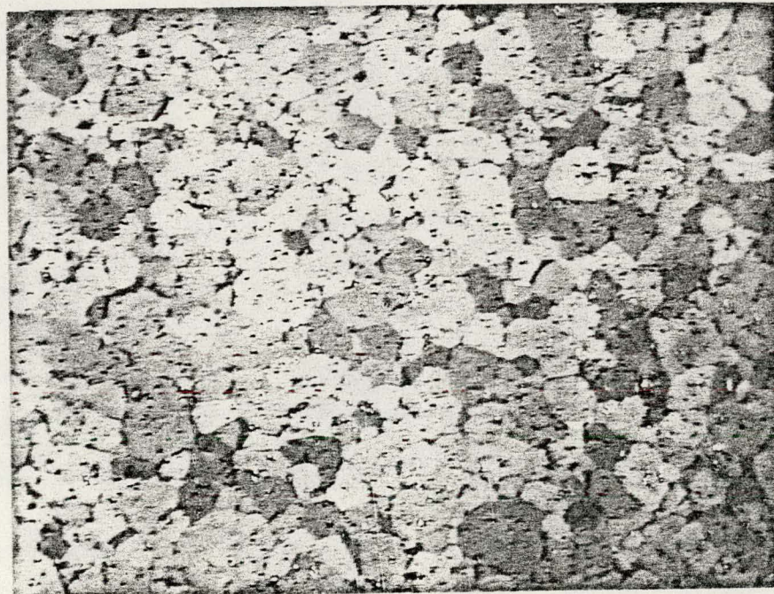
Figure 16. Rod 312-1 transverse cladding microstructure from 0.53 to 0.55 m.
