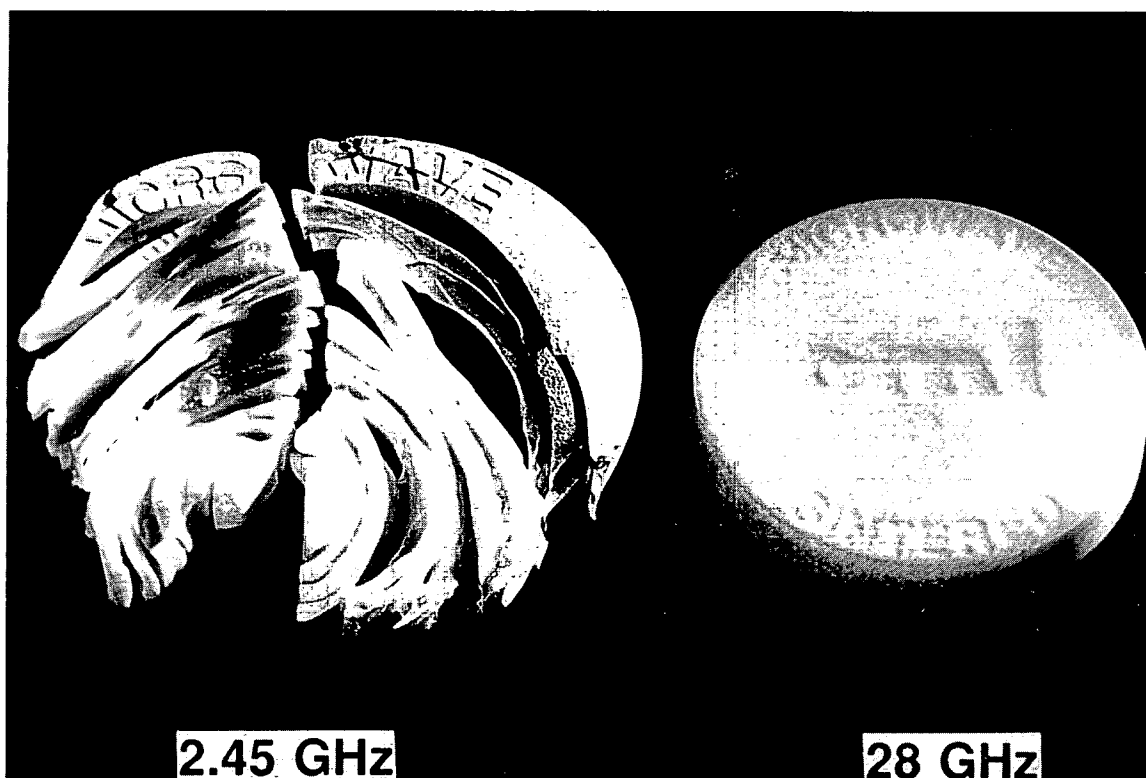
Fig. 12. Striking examples of good and bad microwave-sintered zirconia medallions. The good piece was fired in the ORNL 28-GHz microwave oven for 1 h at 1150°C. During sintering of the bad piece, a hot spot developed that generated differential shrinkage, resulting in large thermal stresses. The stresses produced the final cracking of the part during sintering.
