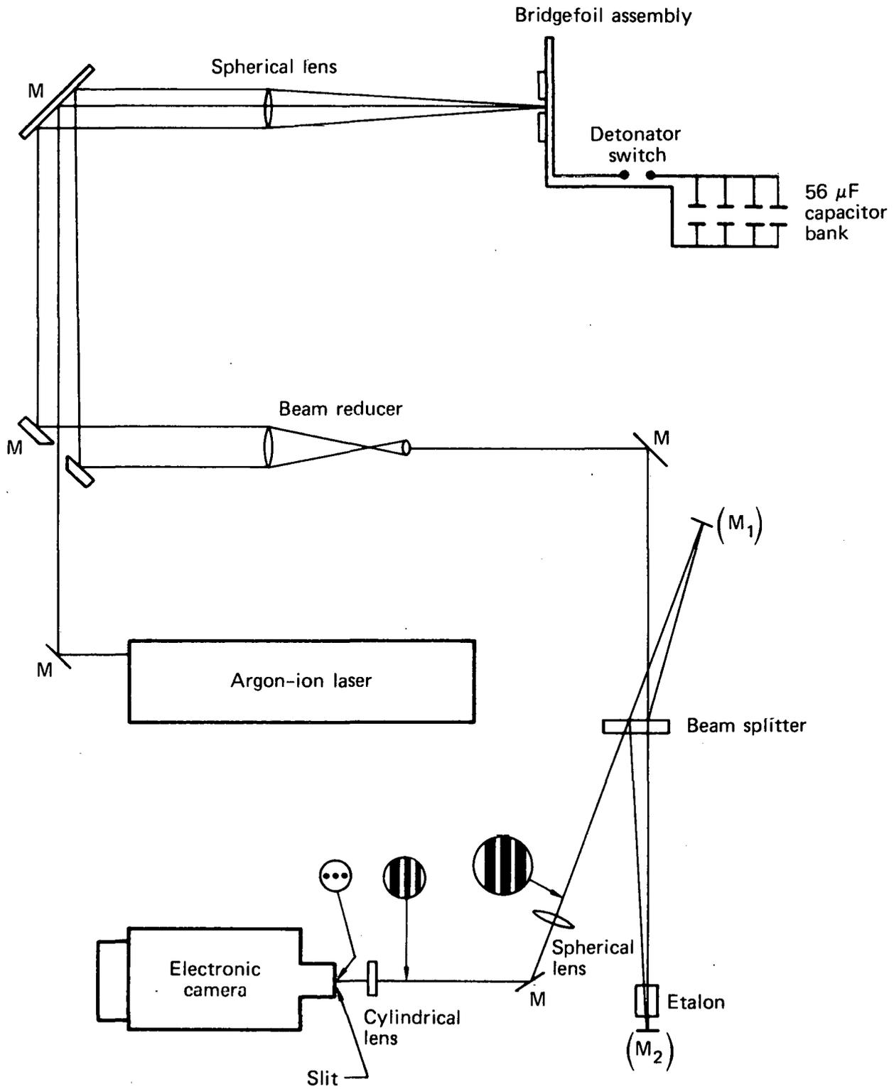
Fig. 1. Experimental setup using an electronic high-speed camera in the streaking mode.
