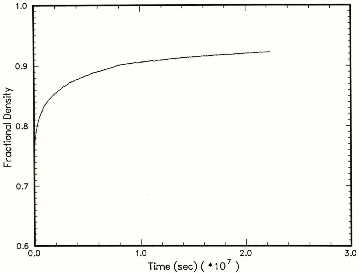
Figure 8: Fractional density-time plot for experiment 08MR89. A subsequent 10.34 MPa stage was run on this specimen, but leaks made the dilatometric data useless. However, the volume change measured by immersion during this stage, and the final measured fractional density are shown in Tables 2 and 3.
