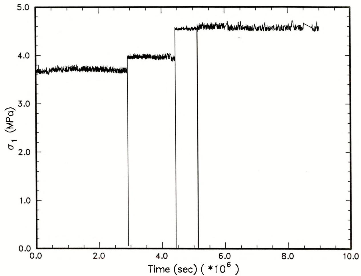
Figure 6: Plot of axial stress *versus* time for shear-consolidation experiment 12OC89.
