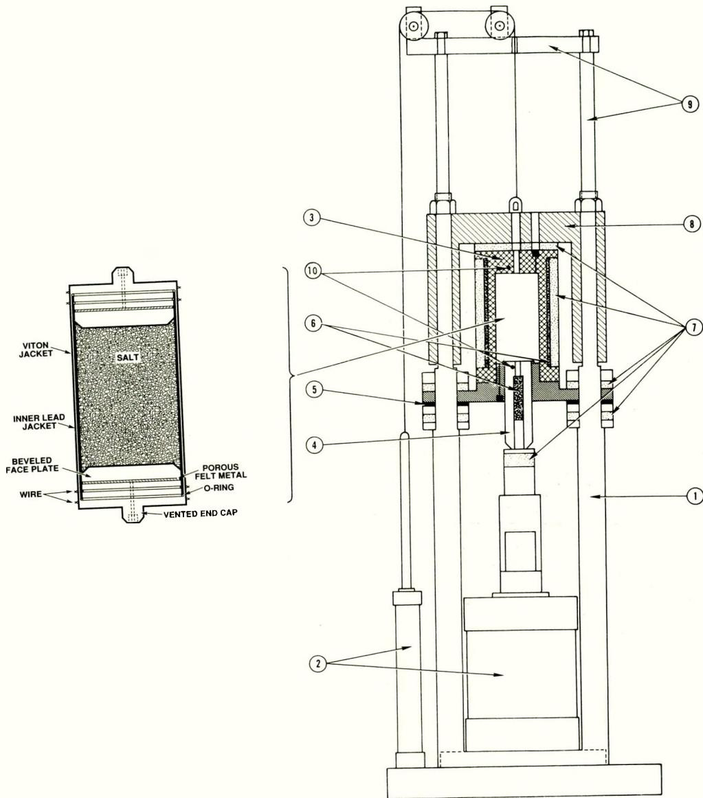
Figure 4: Triaxial testing apparatus designed by W.R. Wawersik and used for our hydrostatic compaction experiments on brine-saturated crushed salt specimens. Numbers on the figure correspond to the following components: (1) tie rods for reaction frame; (2) hydraulic actuators; (3) pressure vessel; (4) deviatoric loading piston; (5) Belleville washers; (6) heaters; (7) insulation; (8) crosshead with guide rods; (9) frame extension/lifting fixture; (10) thermocouple location.
