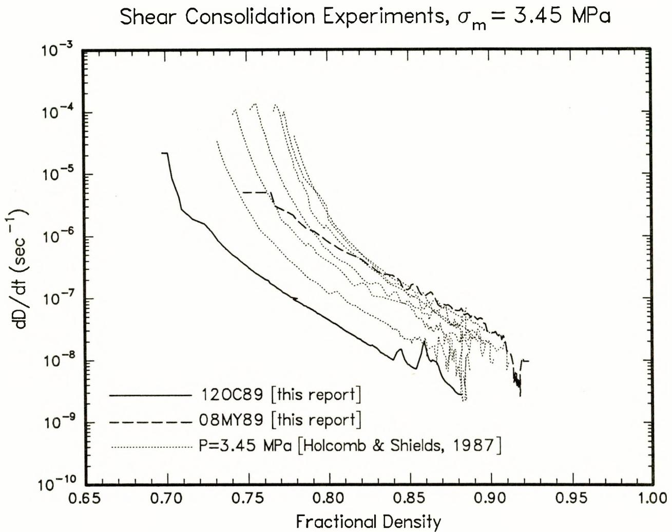
Figure 20: Plot of the time derivative of fractional density *versus* fractional density for our two shear-consolidation experiments, 08MY89 and 12OC89, the dashed and solid lines, respectively. Shown for comparison are results from all of the experiments performed by Holcomb and Shields [1987] at 3.45 MPa on unsaturated, crushed WIPP salt (dotted lines).
