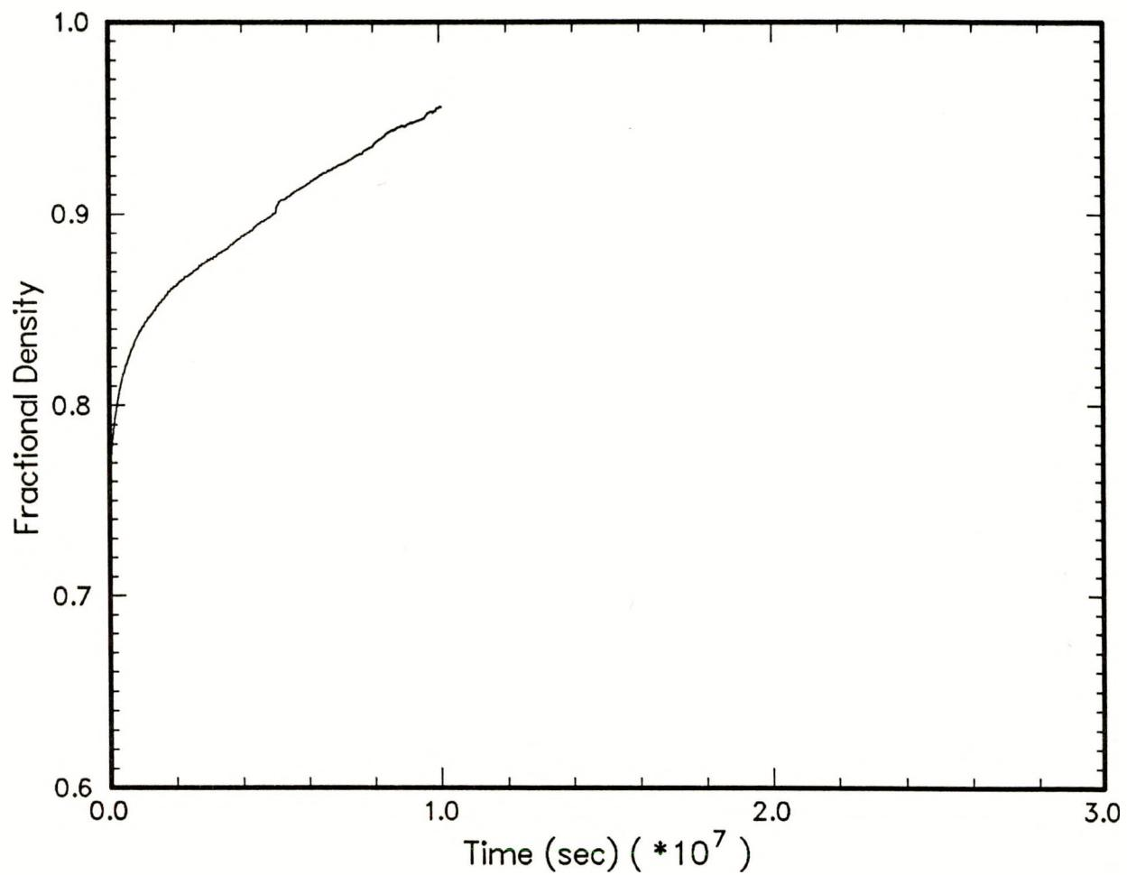
Figure 9: Fractional density-time plot for experiment **20SE89**.
