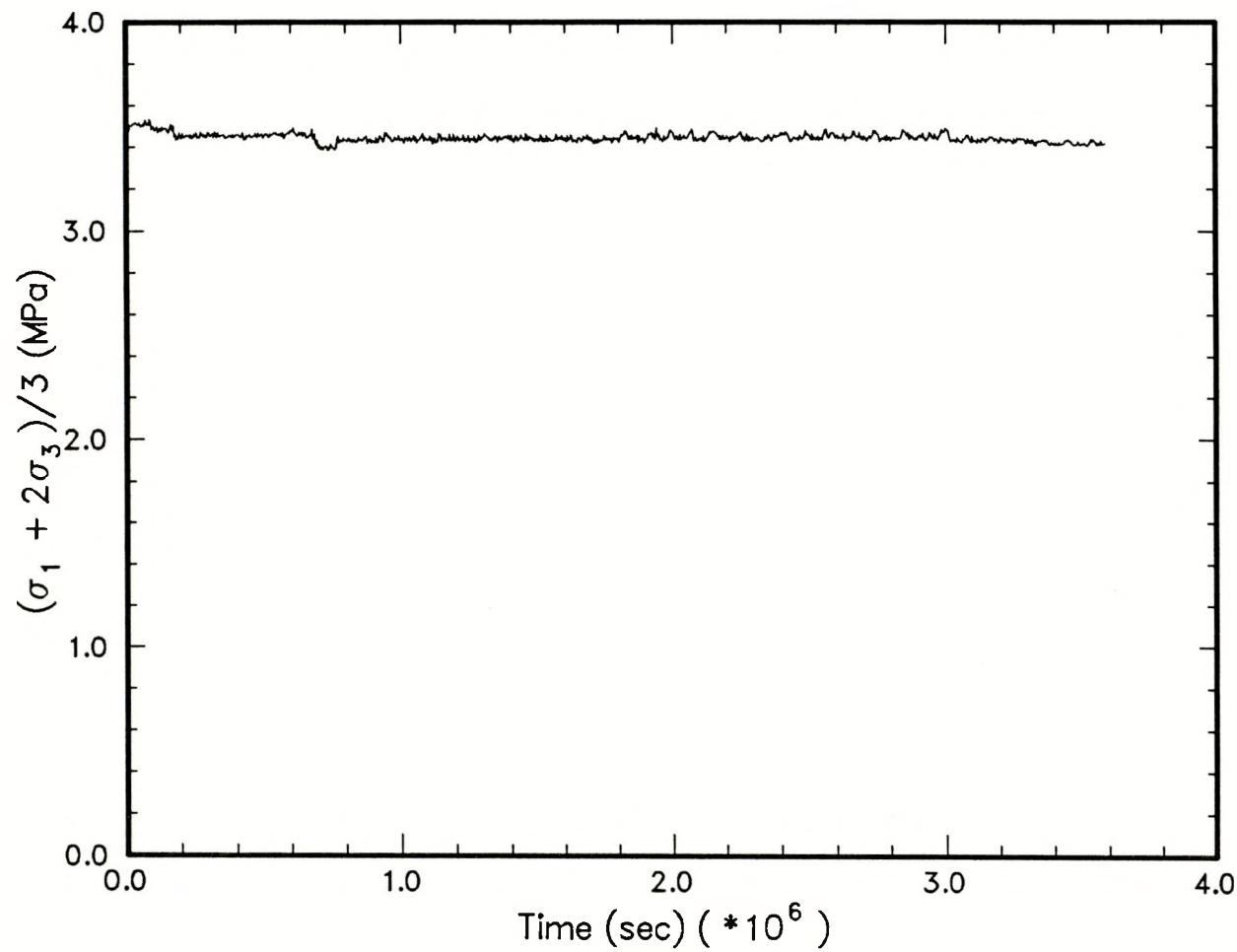
Figure 1: Plot of mean stress *versus* time for shear-consolidation experiment 08MY89.
