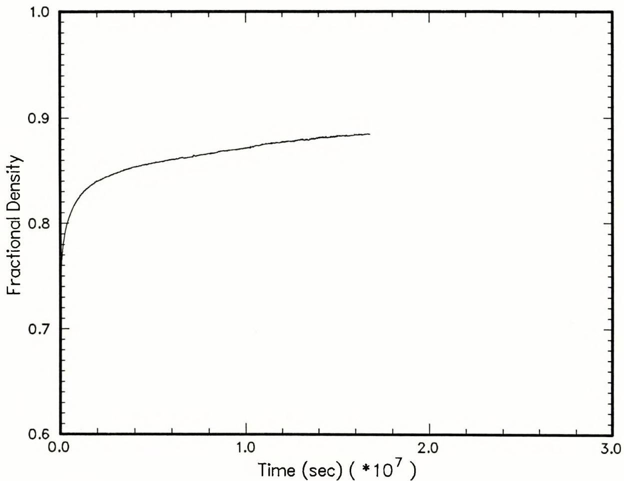
Figure 10: Fractional density-time plot for experiment **18AP89**. An additional stage at 10.34 MPa was run on this sample, but leakage rendered the dilatometric data useless. Measurements made by direct immersion are given in Tables 2 and 3.
