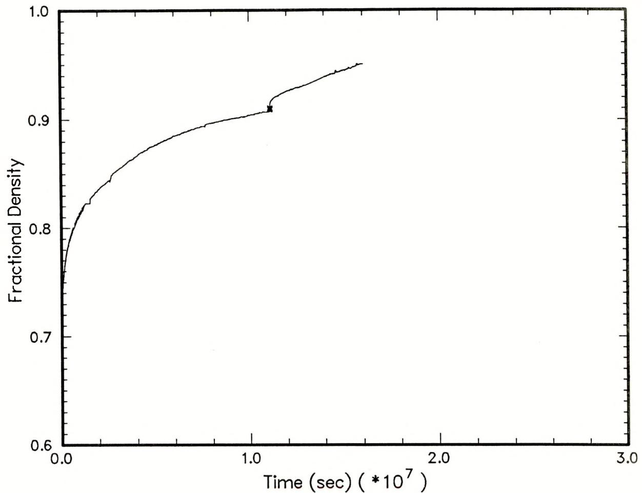
Figure 7: Fractional density-time plot for experiment 09JU88. The nearly-overlying crosses represent (1) the direct volume measurement at the end of the 3.45 MPa stage and (2) the direct volume measurement following quasistatic conditioning prior to the 6.90 MPa creep stage.
