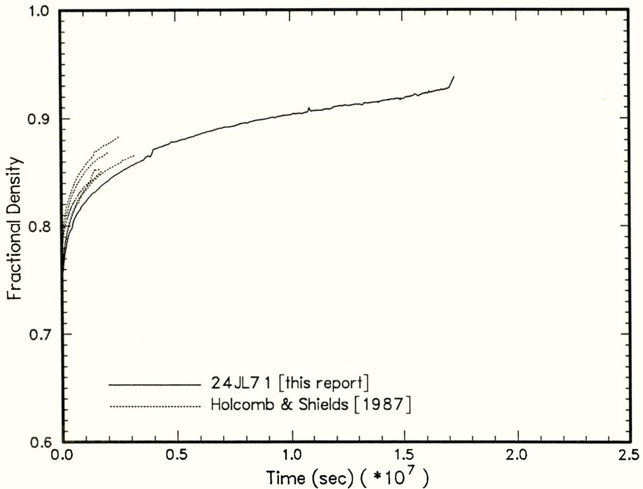
Figure 12: Comparison of experiment **24JL71**,  $P=1.72$  MPa, with tests done by Holcomb and Shields [1987] on unsaturated crushed salt at the same pressure.
