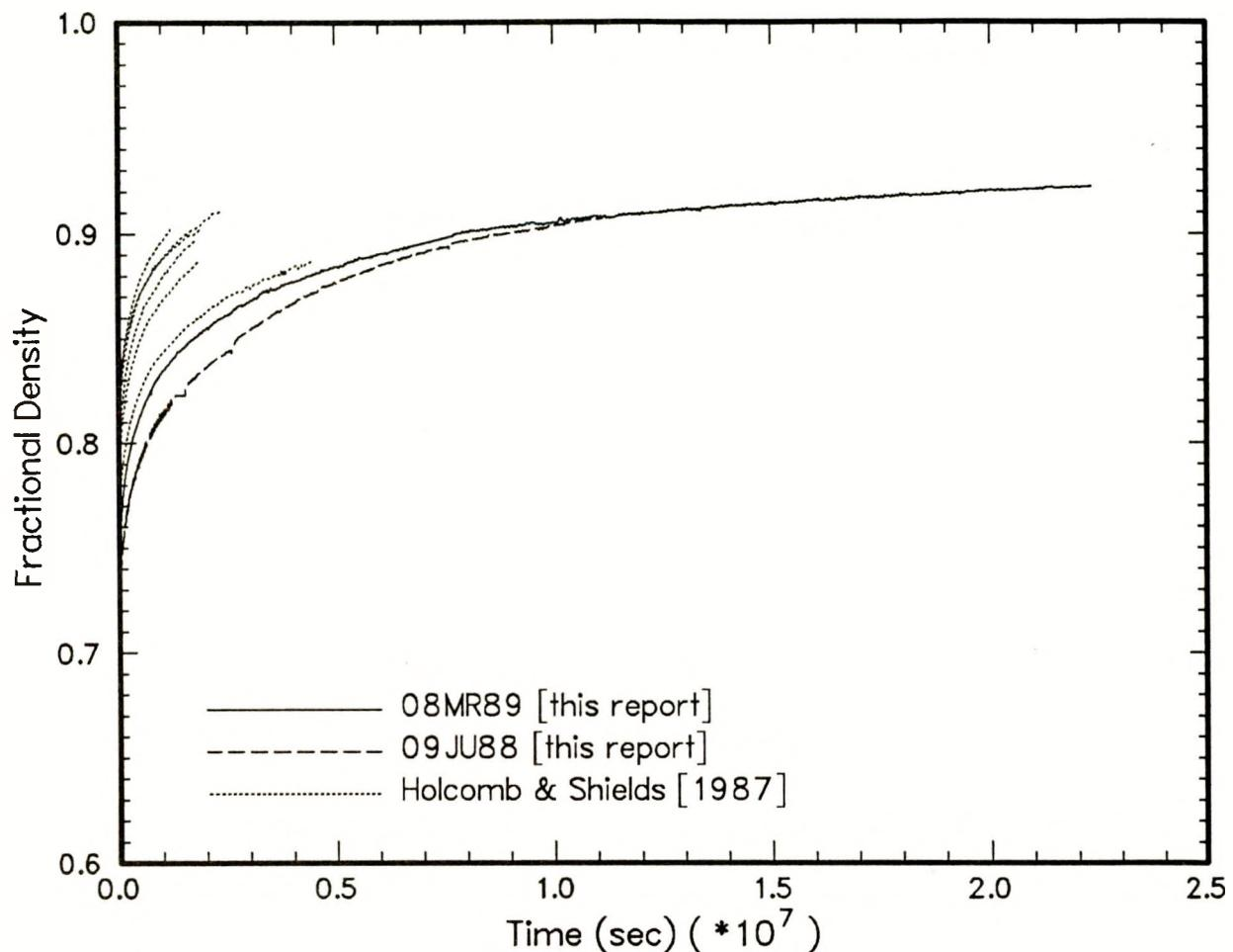
Figure 13: Comparison of experiments 08MR89 and 09JU88,  $P=3.45$  MPa, with tests done by Holcomb and Shields [1987] on unsaturated crushed salt at the same pressure.
