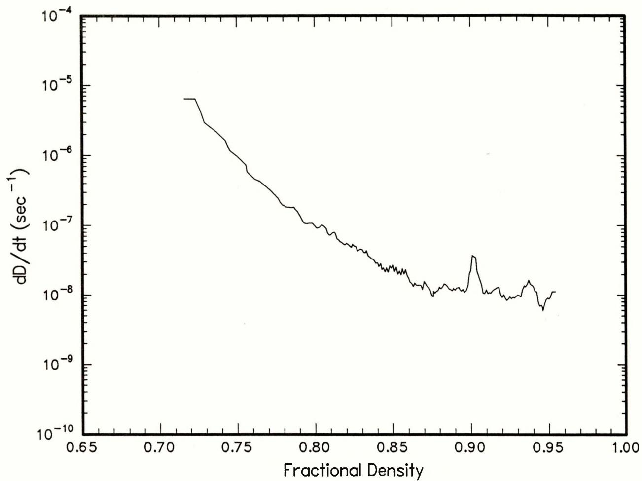
Figure 17: Plot of time derivative of fractional density *versus* fractional density for experiment **20SE89**.
