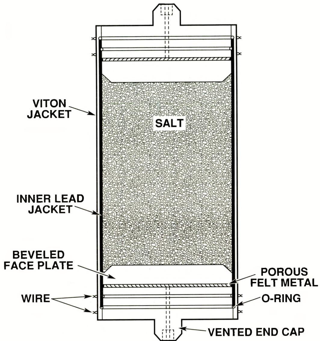
Figure 2: Sample assembly used for crushed salt testing in this study. Two different sizes were used for the hydrostatic and shear-consolidation experiments (see text).
