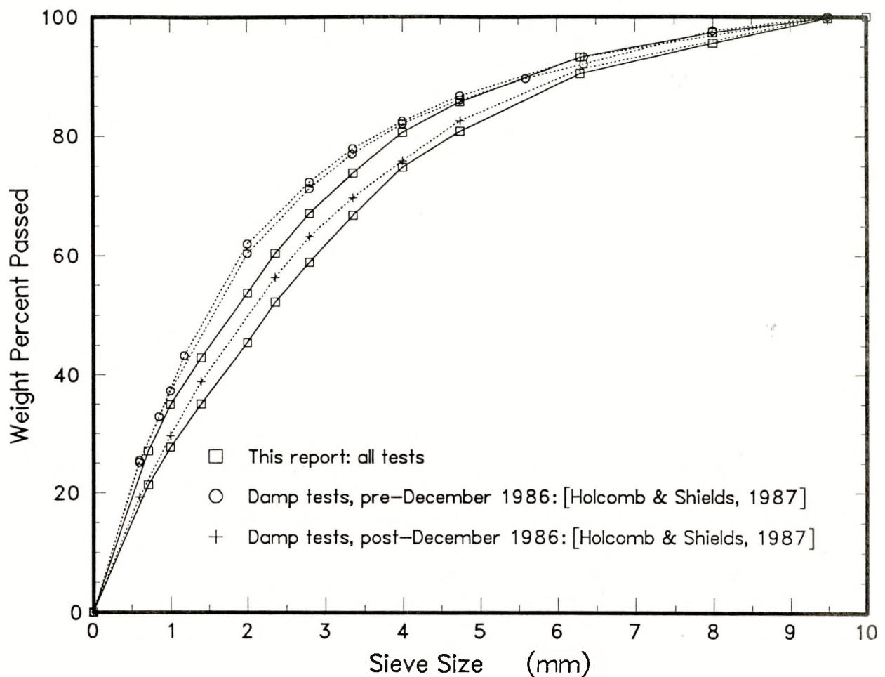
Figure 1: Particle size distribution for the crushed WIPP salt used in this study. Shown for comparison are size distributions for the two crushed salt batches used by Holcomb and Shields [1987]. Our material was drawn from the “post-December 1986” batch, and our results bracket those of Holcomb and Shields.
