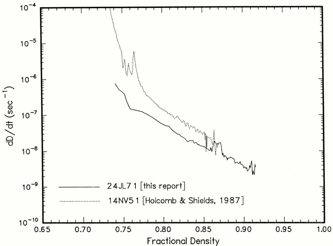
Figure 14: Plot of time derivative of fractional density *versus* fractional density for experiment **24JL71** (solid line). Shown for comparison are data from a representative experiment on unsaturated crushed salt done by Holcomb and Shields [1987] (**14NV51**) at the same pressure, 1.72 MPa.
