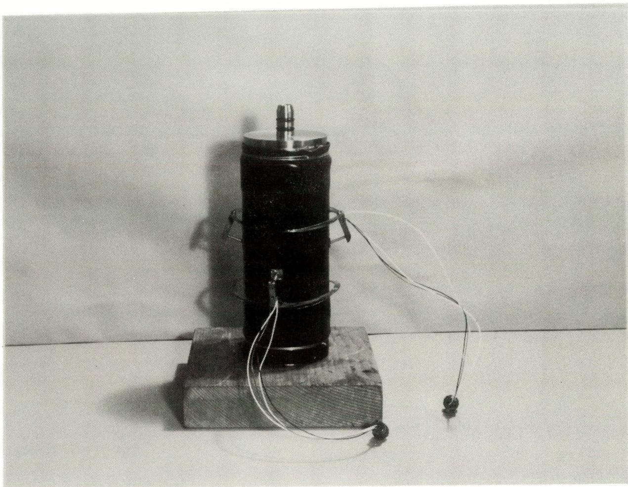
Figure 3: Photograph showing the manner in which disk gauges [Schuler, 1979] are mounted on the outer Viton jacket of the sample assembly. Note that two gauges were mounted across approximately perpendicular diameters.
