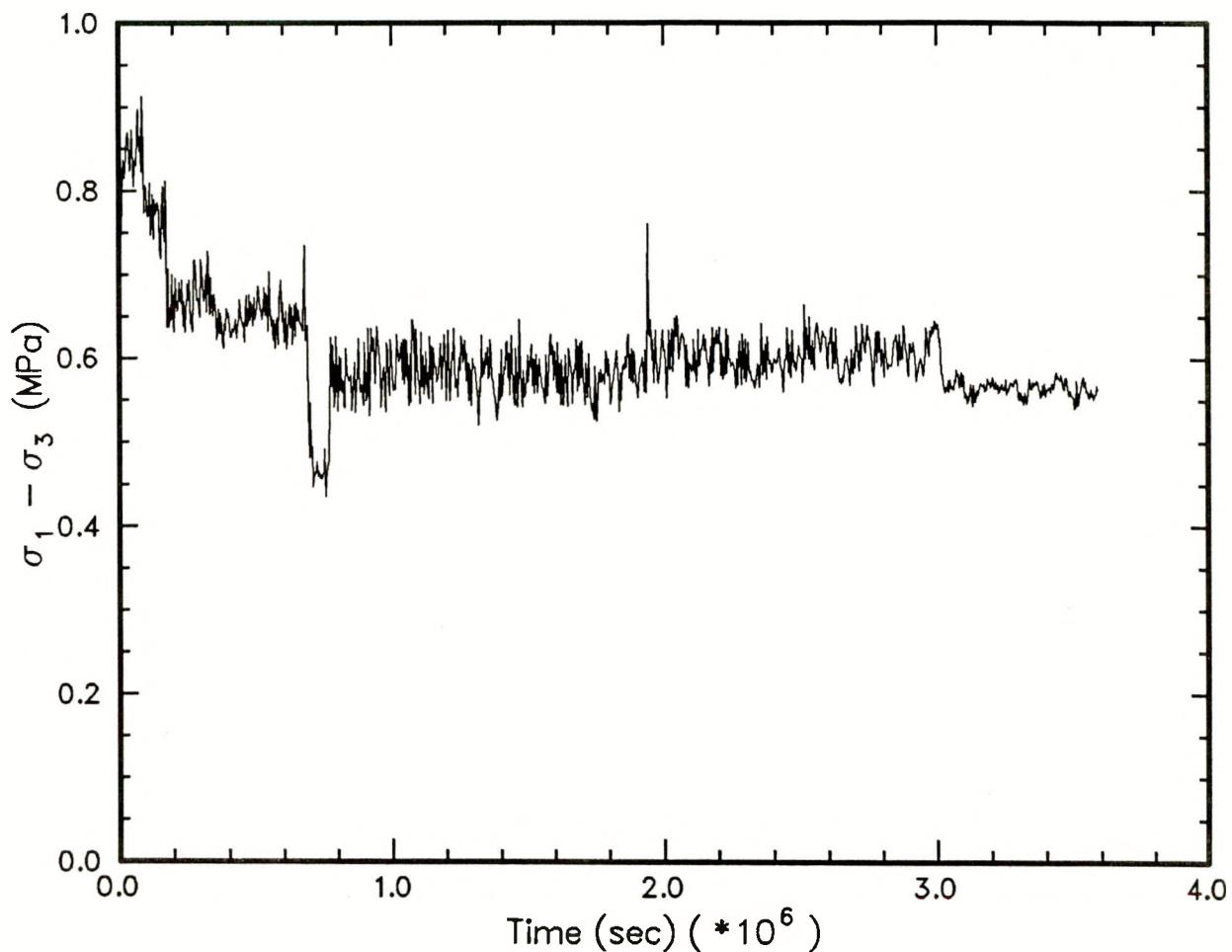
Figure 2: Plot of stress difference *versus* time for shear-consolidation experiment 08MY89.
