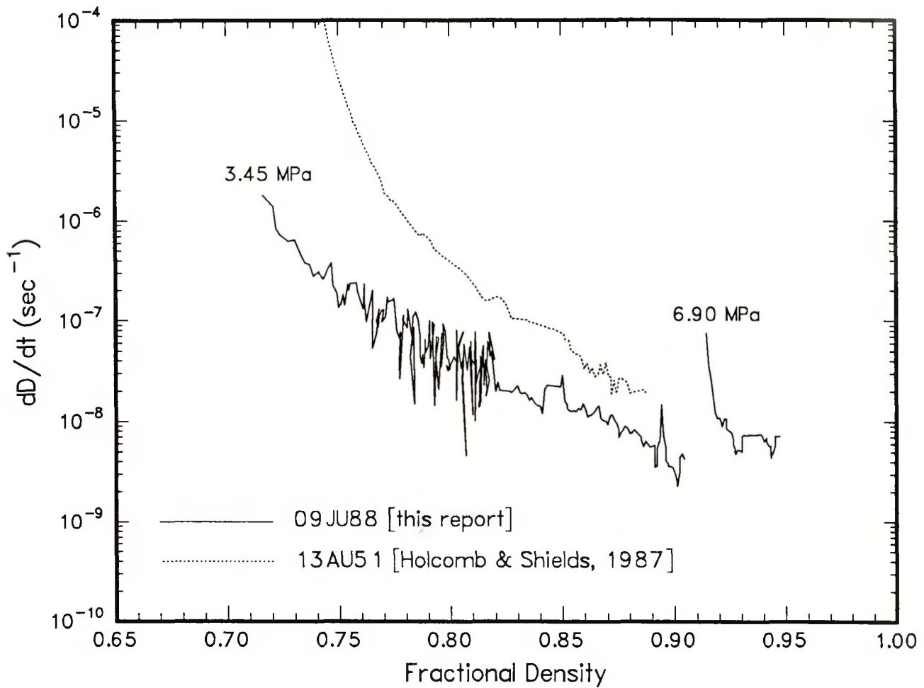
Figure 15: Plot of time derivative of fractional density *versus* fractional density for experiment **09JU88** (solid lines). The break in the solid line represents the change in pressure from 3.45 to 6.90 MPa. Shown for comparison with the 3.45 MPa stage are data from a representative experiment on unsaturated crushed salt done by Holcomb and Shields [1987] at 3.45 MPa (their experiment **13AU51**).
