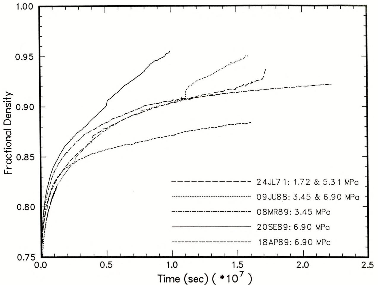
Figure 11: Summary plot of fractional density-time data for hydrostatic compaction experiments on brine-saturated crushed WIPP rock salt. See text for discussion.
