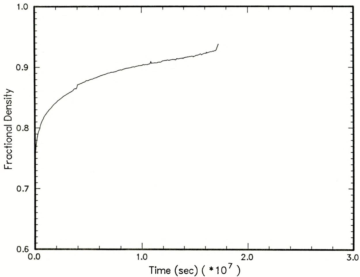
Figure 6: Fractional density-time plot for experiment **24JL71**. The final upturn in the plot is where accidental overloading occurred.
