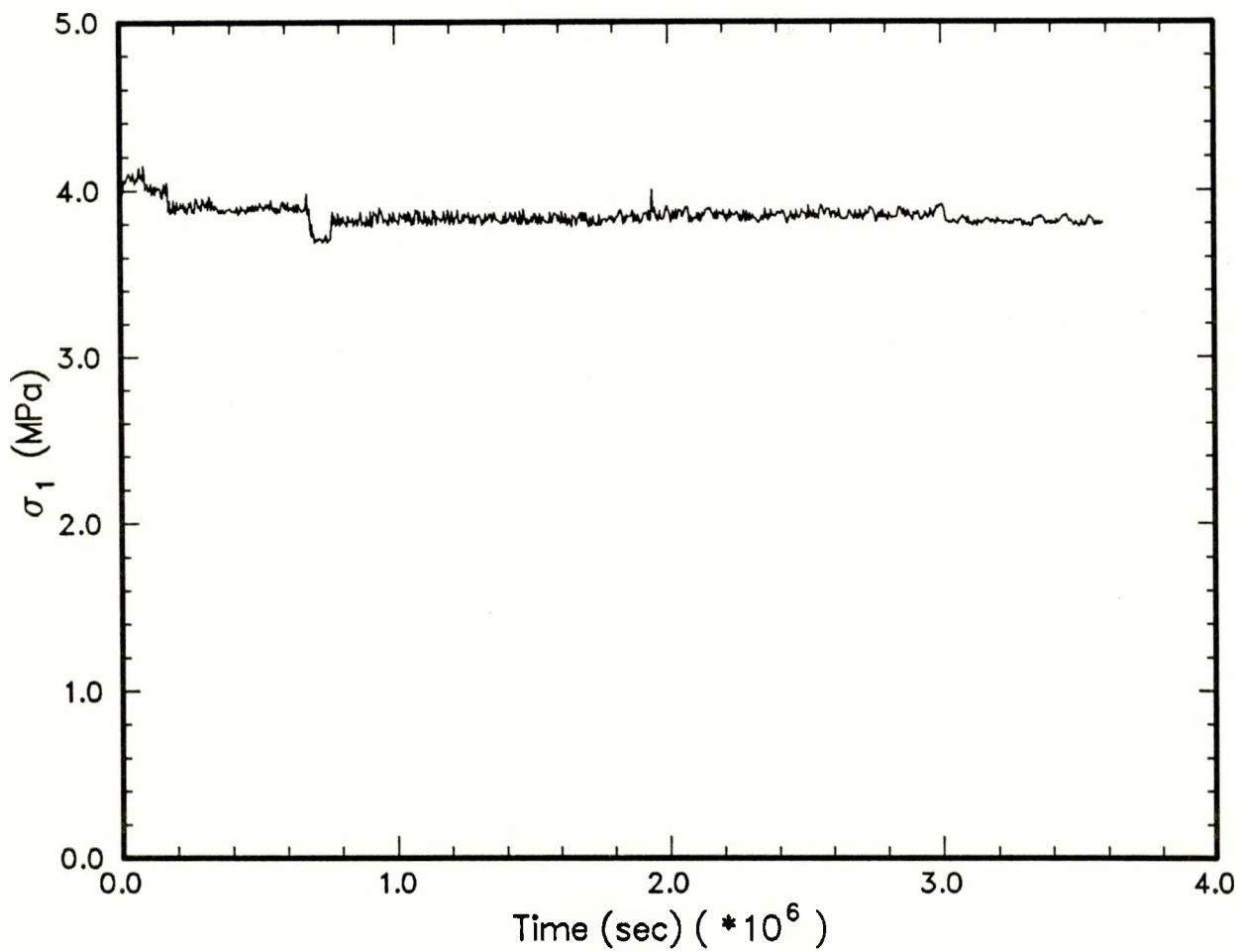
Figure 3: Plot of axial stress *versus* time for shear-consolidation experiment 08MY89.
