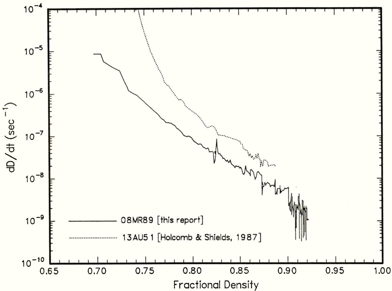
Figure 16: Plot of time derivative of fractional density *versus* fractional density for experiment 08MR89 (solid line). Shown for comparison are data from a representative experiment on unsaturated crushed salt done by Holcomb and Shields [1987] (13AU51) at the same pressure, 3.45 MPa.
