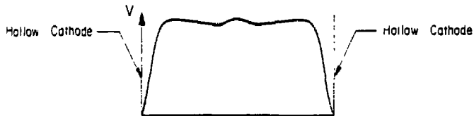
(b) Potential Distribution Across the Diameter of the Hollow Cathode
