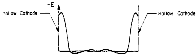
(c) Electric Field Distribution Inside the Hollow Cathode
