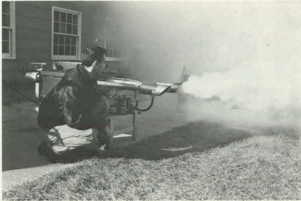
Figure 12. Smoke generator emitting oil-fog smoke from one nozzle.
