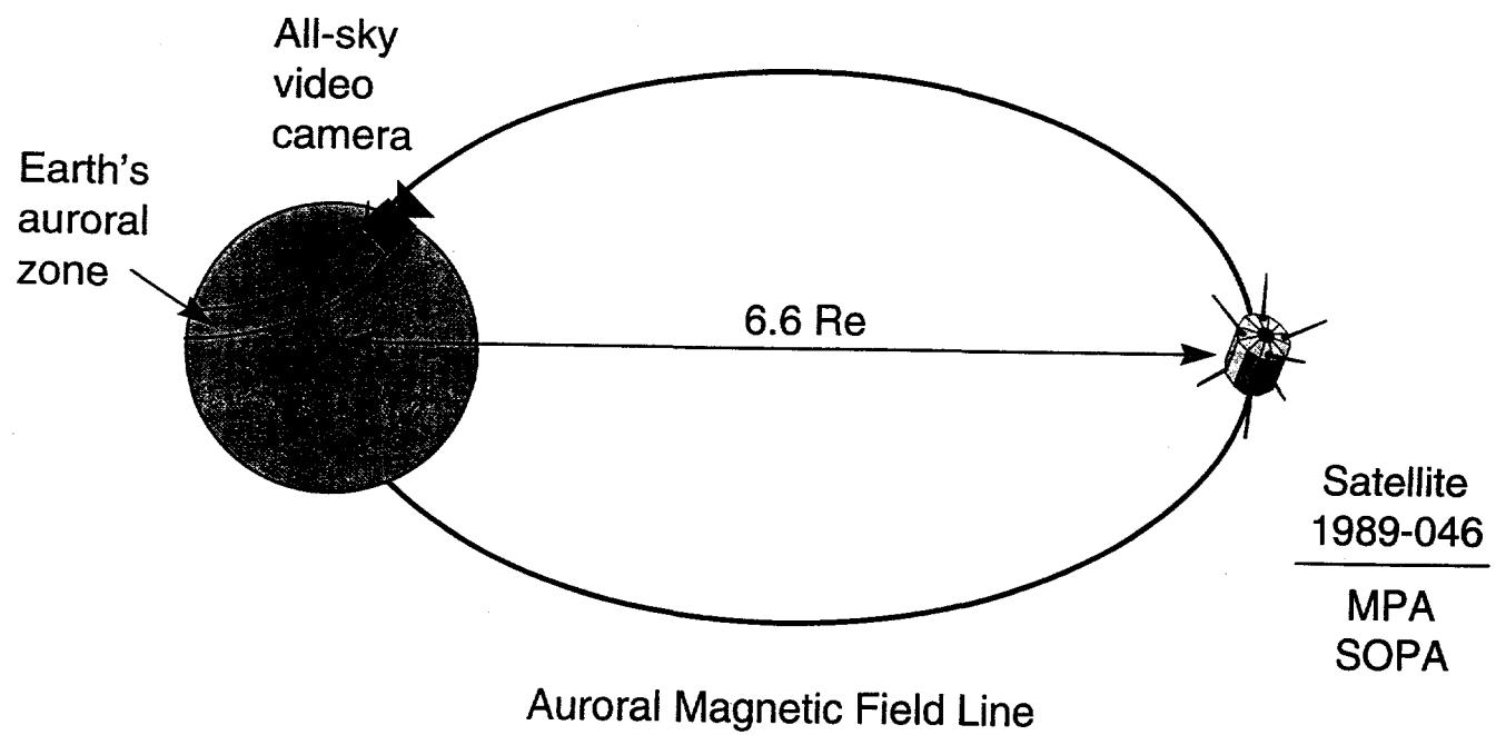
Figure 1. Experimental configuration showing the magnetic field-line connectivity of the ground-based all-sky video camera and the geosynchronous satellite 1989-046.
