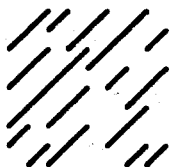
Random Fractures or Joints
