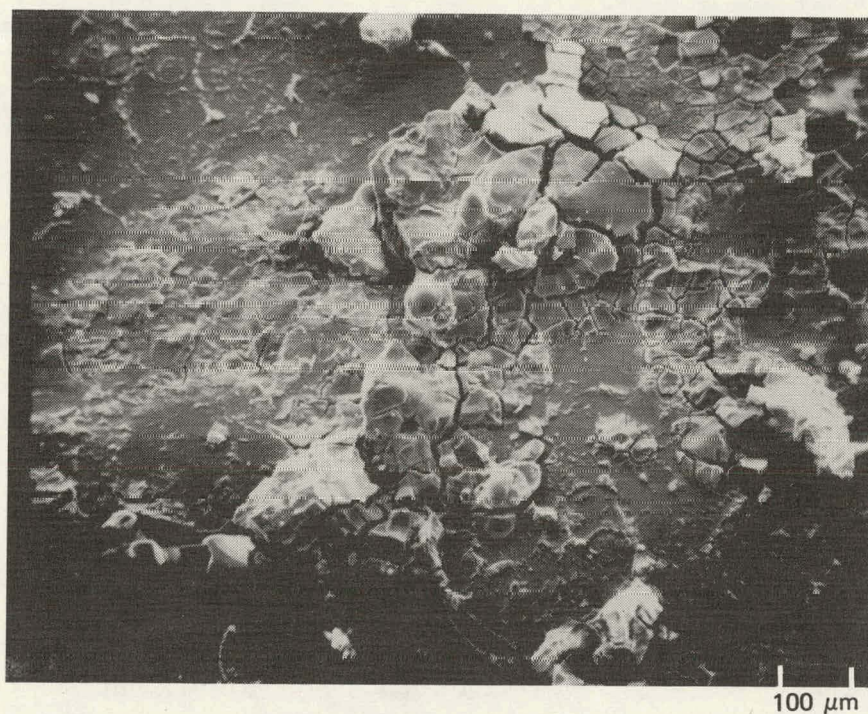
B. 100X magnification of residual soil layer of a cleaned specimen exposed 12 months at Stauffer Chemical Co.
