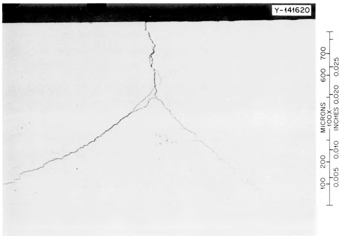
Fig. 8.2. Longitudinal section of 1080 steel wire strained in 0.1M H_2S at 21°C.
