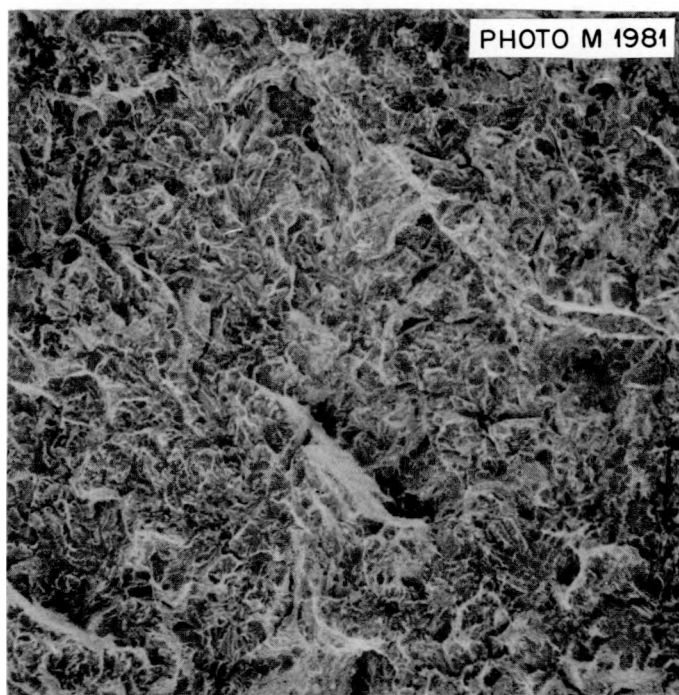
Fig. 6.11. Scanning electron microscopy photomicrographs of representative areas from the fracture surface that occurred as a consequence of TSE-3. The fracture exhibits a predominately cleavage mode with small areas of dimple fracture.
