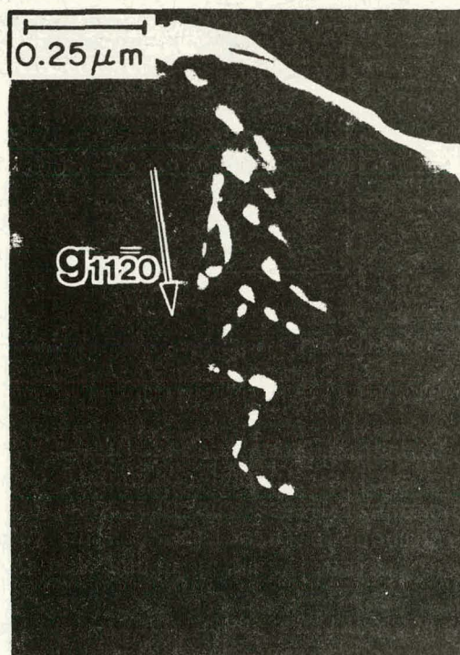
Fig. 3. (11\bar{2}0) dark-field transmission electron microscope image of nonbasal dislocations from the (10\bar{1}0)[1\bar{2}10] and (0\bar{1}10)[\bar{2}110] slip systems in hexagonal ice. Film orientation: [3\bar{3}02] .
