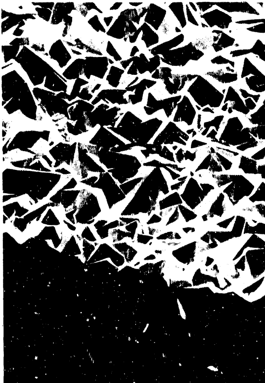
A film dominated by {111} faces has been broken in half to reveal the columnar structure created during its early growth, as shown in this micrograph.
