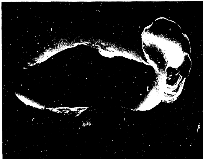
This award-winning scanning electron micrograph by Mukund Rao and Jim Keiser shows a crater produced on an aluminum surface by the impact of a single spherical particle of tungsten carbide propelled at 661 m/s by helium in a light-gas gun.
