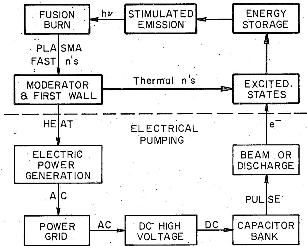
Figure 1. Comparison of nuclear and electrically pumped laser fusion concepts. Additional steps required for electrical pumping are shown below the dashed line.
