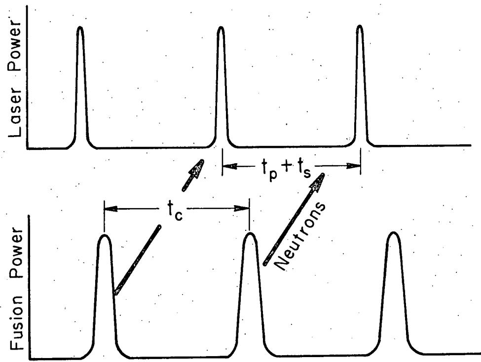
Figure 2. Timing of fusion laser pulse and pellet burn.
