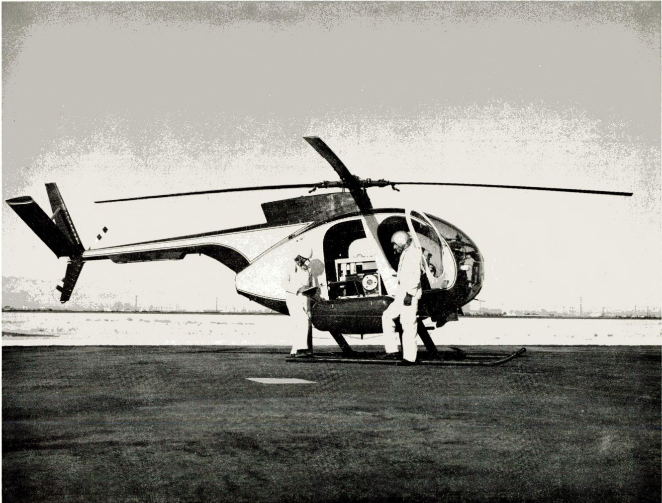
Figure 4. The Hughes H-500 helicopter is operated by a pilot and a navigator. The latter also operates the REDAR system shown in the rear compartment. Detector pods on the left and right each contain ten sodium iodide detectors.
