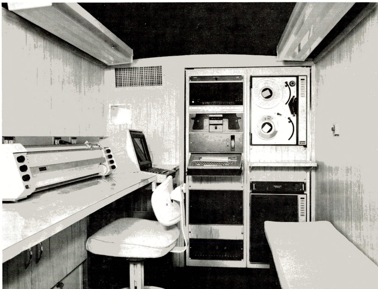
Figure 5. The heart of the REDAC system is a NOVA 840 computer. Sophisticated software routines allow preliminary isopleths to be prepared in the field. Gamma spectra may be obtained immediately after the aircraft returns from a mission.
