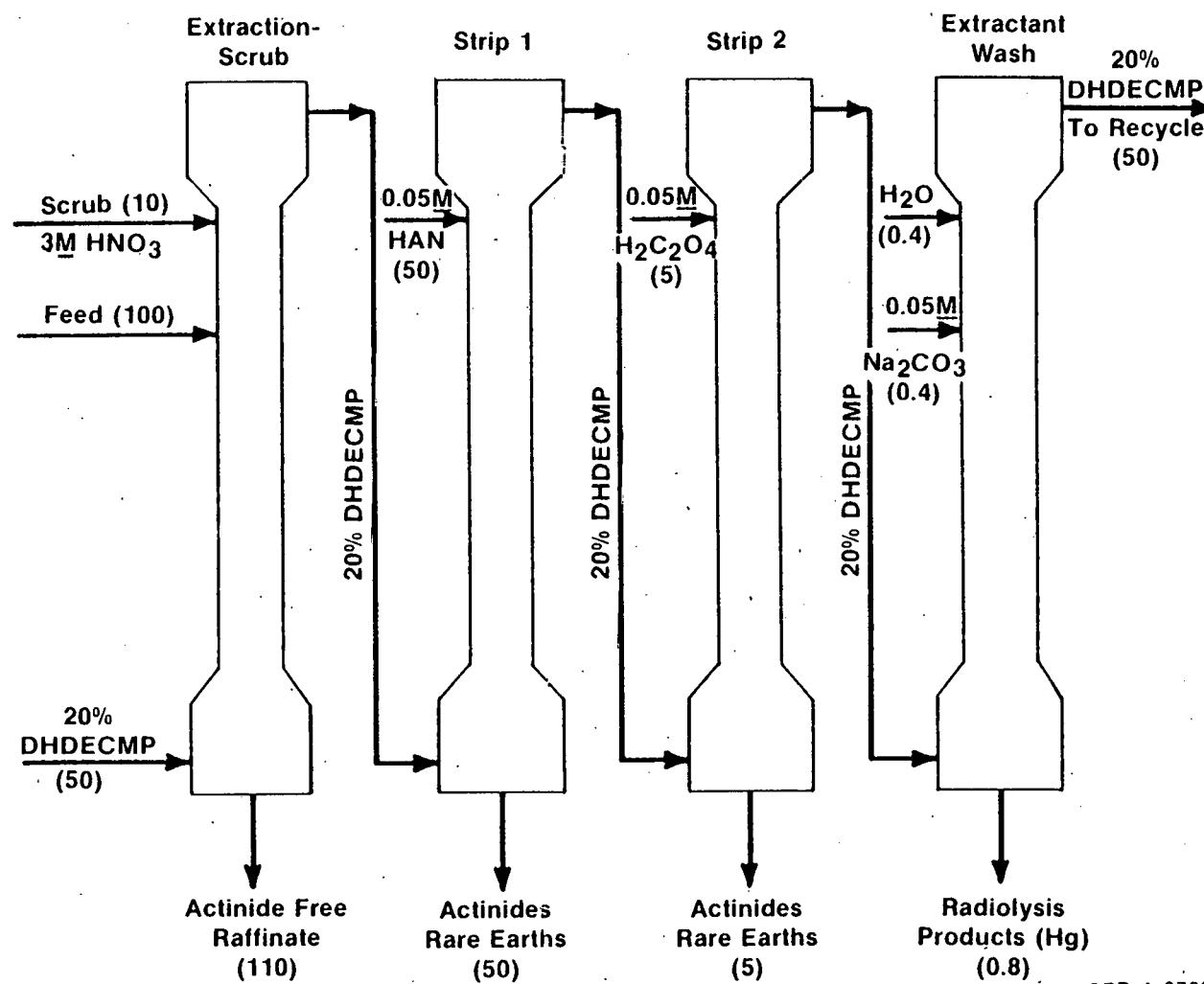
FIGURE 3. PARTITIONING MIXER-SETTLER SCHEMATIC
