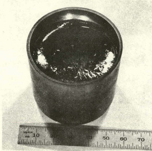
Fig. 4. Silicon Directionally Solidified (Bottom to Top) in a Vitreous Carbon Crucible
