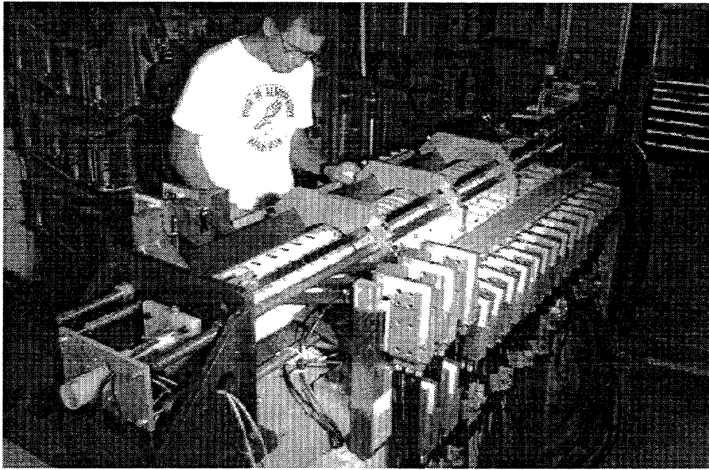
Figure 6.5 Line of solenoidal magnets (30 at 100 kG, 5 at 240 kG).
