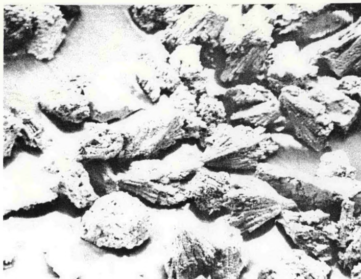
(a) Powder used for plasma spraying (1700X) Fired to 1800°C, 2 hrs.; Screened to -150 + 325 mesh.
