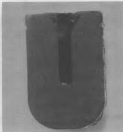
FIGURE 4.1. NiO-NiFe 2 O 4 -17% Cu round-bottomed anode used in Test 59 (Anode 115-24). Deposit on surface is frozen electrolyte.
