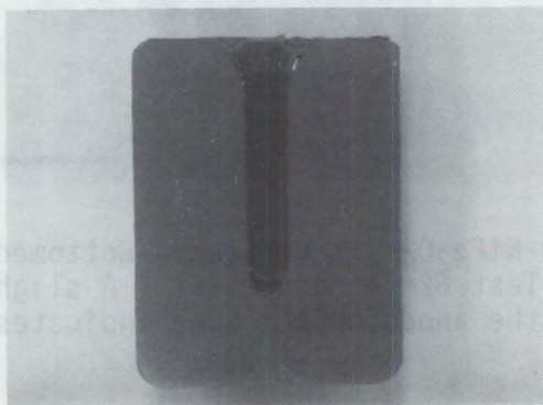
FIGURE 4.5. \text{NiO-NiFe}_2\text{O}_4\text{-Cu-Ni-Al} Square-Bottomed Anode Used in Test 63 (Anode 104-2). The anode showed a slight amount of discoloration across the entire anode surface.
