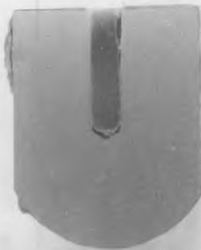
FIGURE 4.8. \text{NiO-NiFe}_2\text{O}_4\text{-Cu-Ni-Al} Round-Bottomed Anode Used in Test 66 (Anode 133-2). This anode showed a halo of discoloration around the perimeter, which is visible at the top of the anode.
