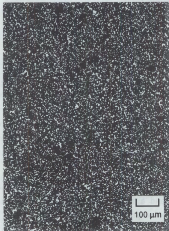
FIGURE 5.10. \text{NiO-NiFe}_2\text{O}_4\text{-Cu-Ni-Al} Cermet Anode (24 wt% Cu, 3 wt% Ni, 1 wt% Al). The as-sintered density was 6.16 \text{ g/cm}^3 .
