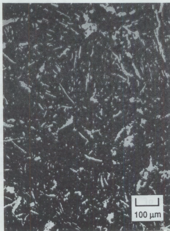
FIGURE 5.6. Anode from PNL Vibration-Milled Oxide, \text{NiO-NiFe}_2\text{O}_4 -17% Cu. Density 6.18 \text{ g/cm}^3 .
