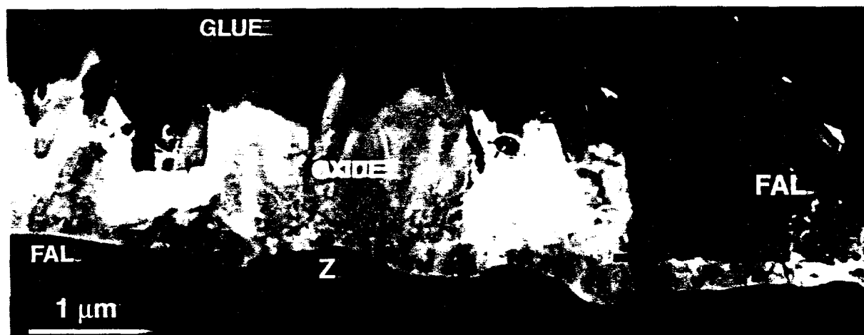
Fig. 7. STEM annular dark-field of coated-and-oxidized (96h at 1000°C) FAL. The location of the original coating is indicated by the arrow.
