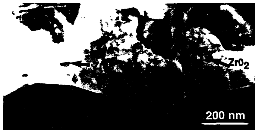
Fig. 8. Annular dark-field STEM image of cross-section through scale showing ZrO_2 particles within the scale.
