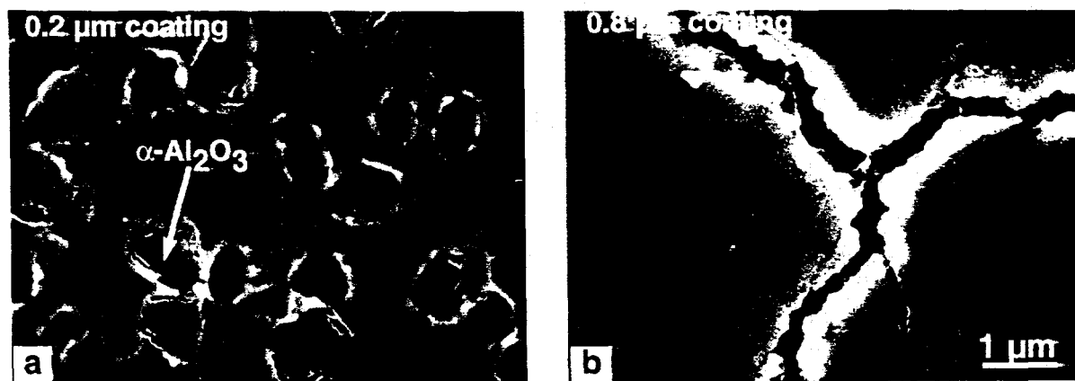
Fig. 2. SEM plan-views of the heat-treated coatings after 2 h in He at 1000°C. (a) 0.2 \mu\text{m} coating, revealing the scale/metal interface (b) 0.8 \mu\text{m} coating, revealing the gas/scale interface.
