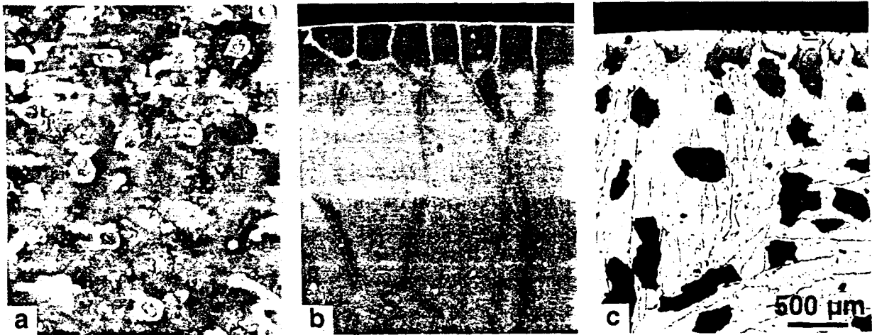
Fig. 9. SEM plan-view images of a) René N5, b) NCA-S and c) NCA-H after oxidation for 100 h at 1200°C.
