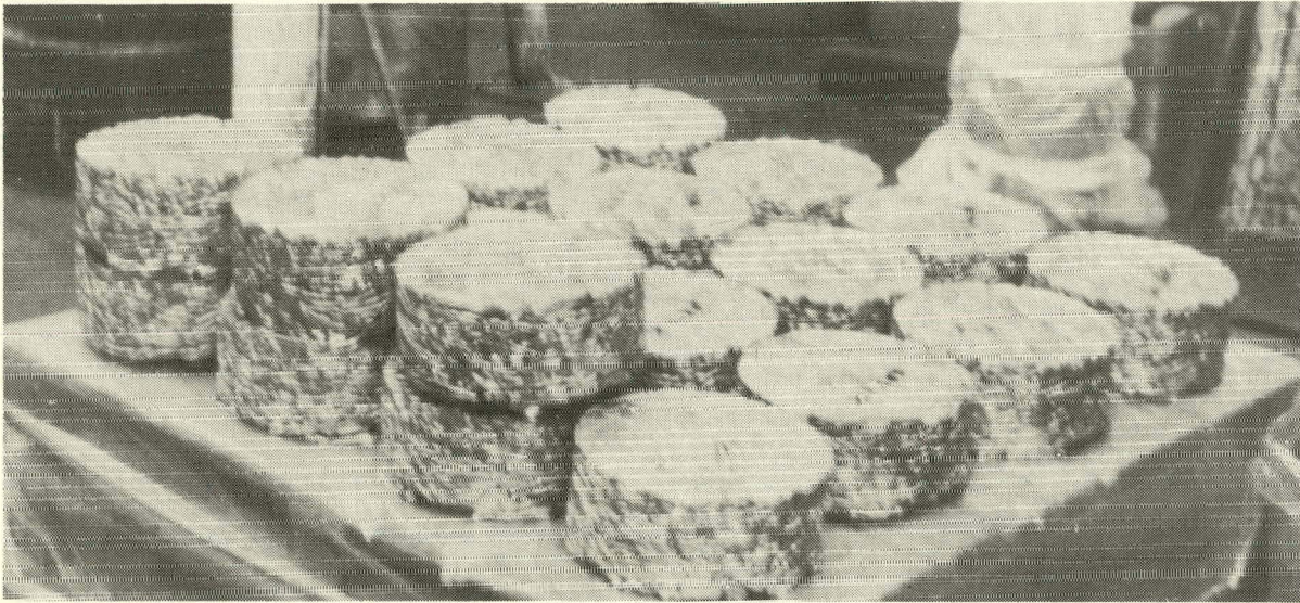
Fig. 5. Zircaloy Tubing Compacts Prepared by Mechanical Compaction (courtesy Teledyne Wah Chang Albany Co., Albany, Oregon)
