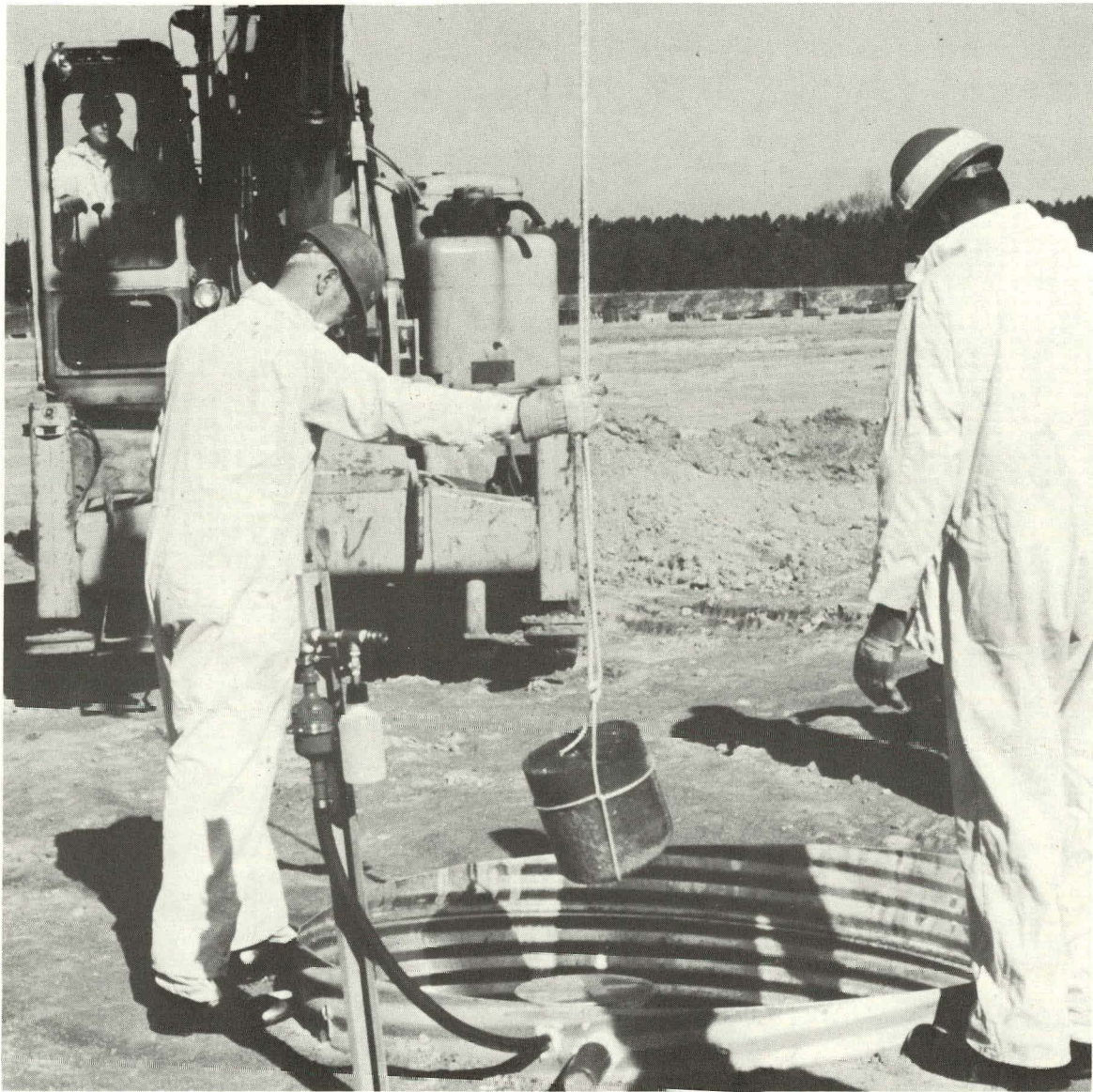
Figure 10. PITC specimen being lowered into lysimeter.
