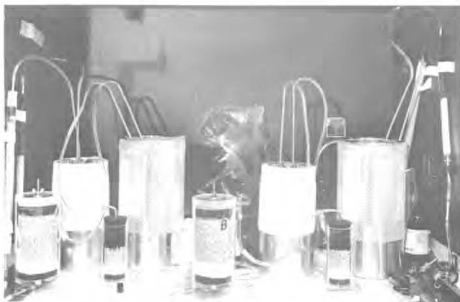
FIGURE 10. Activated Carbon Canisters in Dry Ice/Alcohol Bath Used for Trapping Radon During Laboratory Tests
