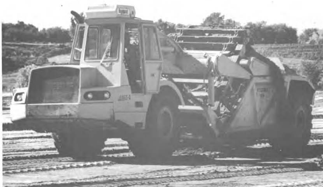
FIGURE 16. Paddle Wheel Earth Mover Removing Overburden
