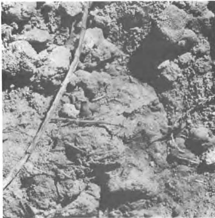
FIGURE 42. Salts Transporting to the Surface of Grand Junction Tailings on Bank Near Colorado River - December 1979
