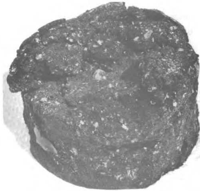
FIGURE 40. Core Sample Taken from the Admix Seal Showing Poor Particle Coating
