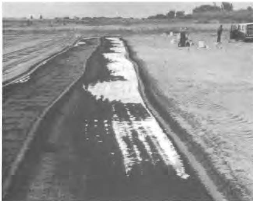
FIGURE 21. Results of Single-Pass, \sim 9 \text{ wt\%} Asphalt Emulsion Application - Poor Mixing
