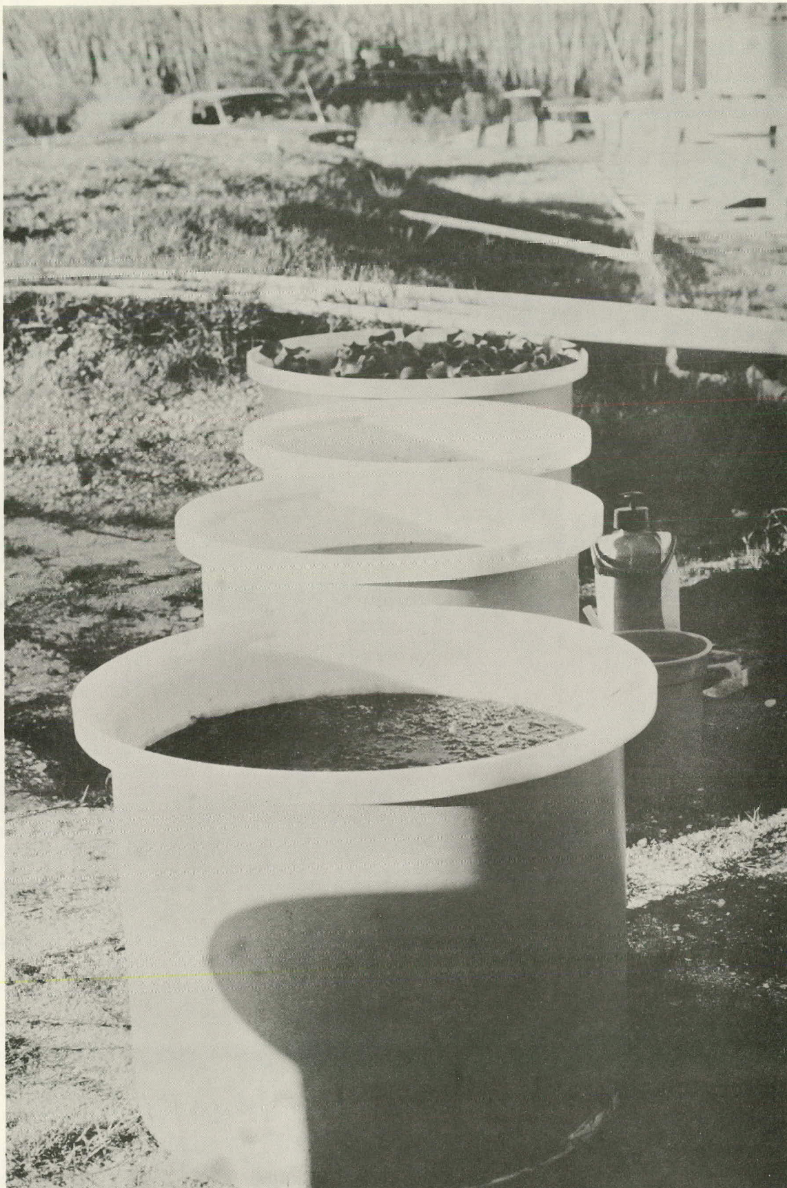
Figure 5. Stagnant cultures of freshwater macrophytes for measuring evapo-transpiration water loss.
