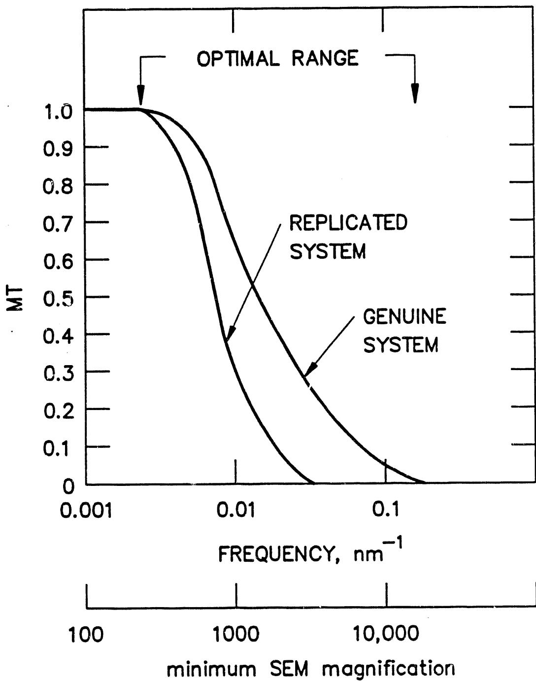
Figure 10. MTF Optimized Magnification and Features
