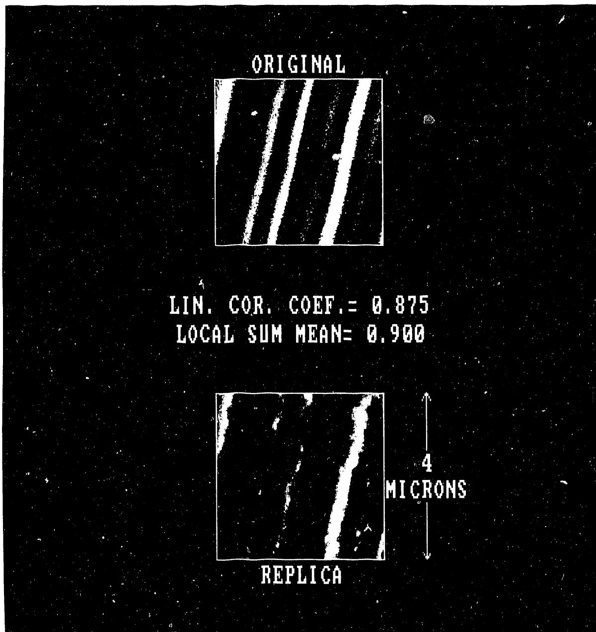
Figure 2b. Original-Replica Image Comparison Using Linear Correlation Coefficient and Local Sum Mean
