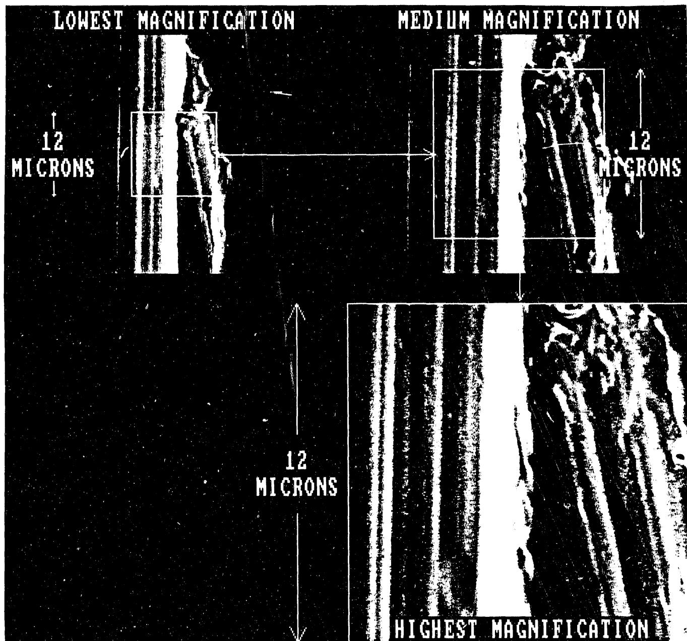
Figure 13. Same Casting Imaged at Magnifications of 1000, 2000, and 4000
