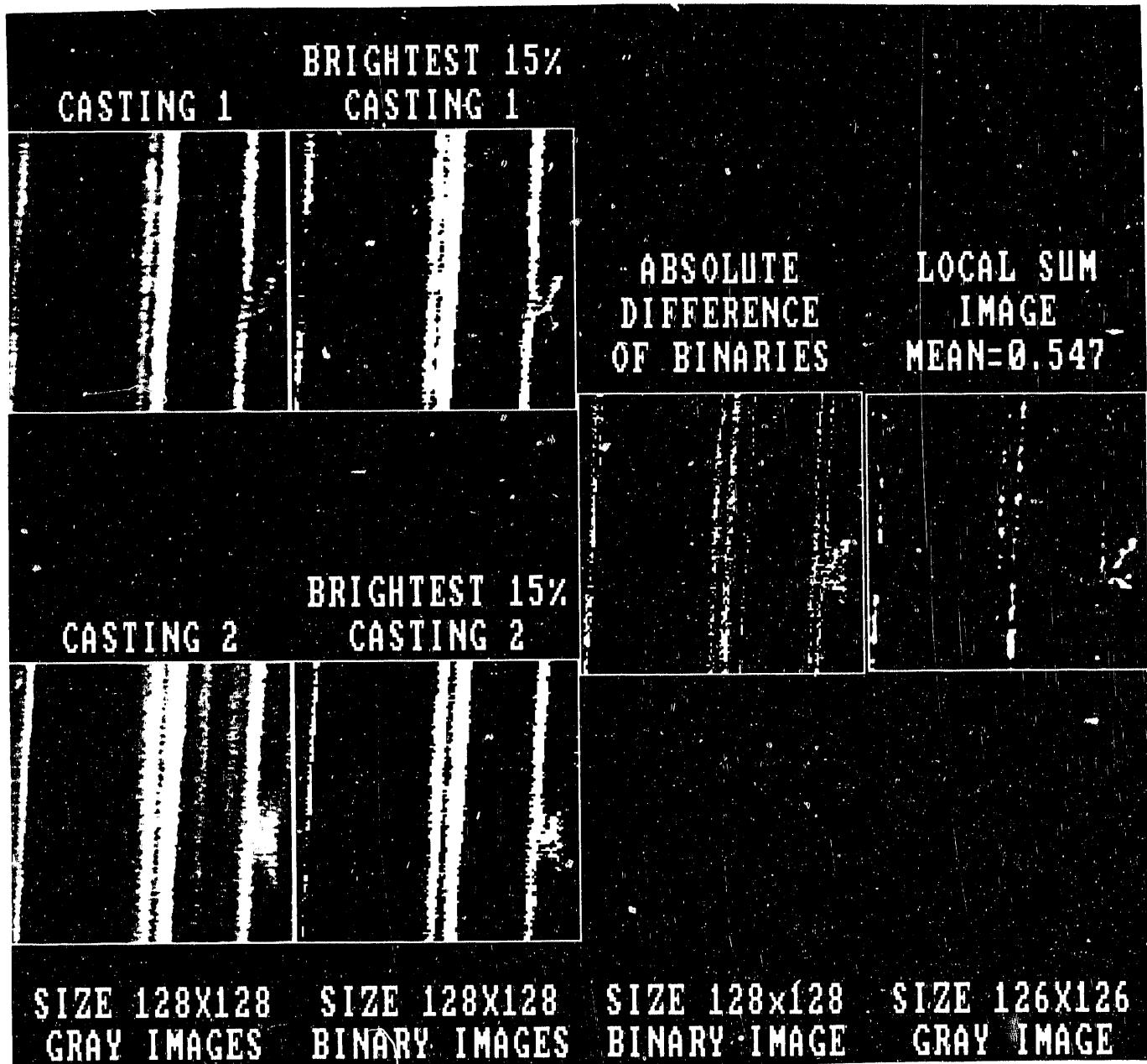
Figure 5. Second Illustration of Steps in Calculating the Local-Sum Image
