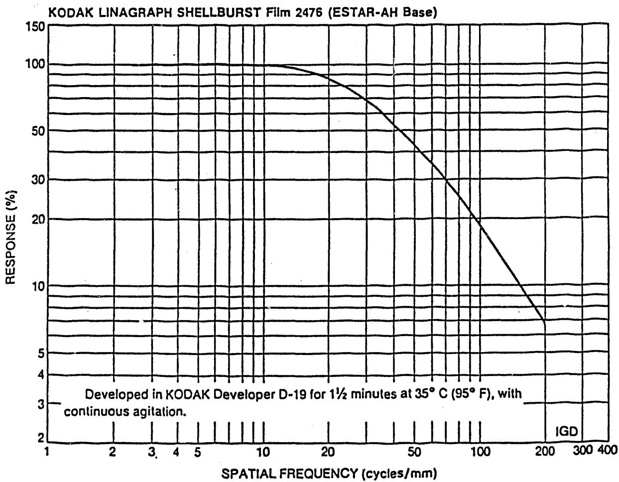
Figure 7. Sample MTF Curve for Photographic Film
