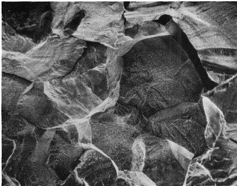
Figure H-65. Fracture Surface of Specimen SS-10 as Seen Near the Sides of Specimen, 100X
