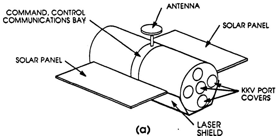
Figure 1. Calculational Model of the Space Based Interceptor Weapon Platform
